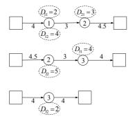
Fig. 2.5. Solution of the MCVRP.
