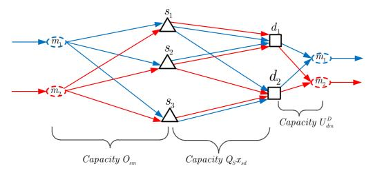
**Fig. 5.1.** An example of an instance for maximum multi-commodity flow.
