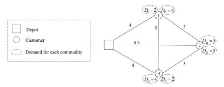
Fig. 2.1. An instance of VRP with two commodities.
