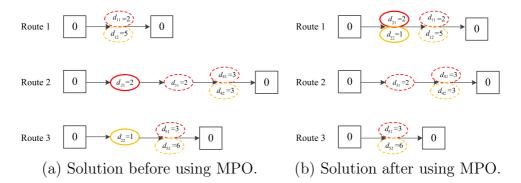
Fig. 3.8. MPO for reassigning commodities.
