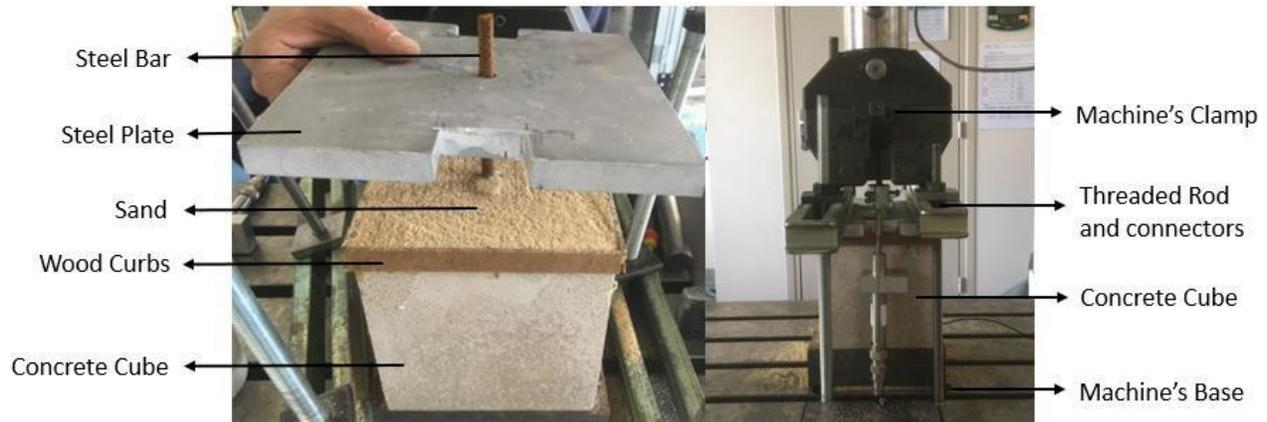
Figure 8: Pull-out testing system
