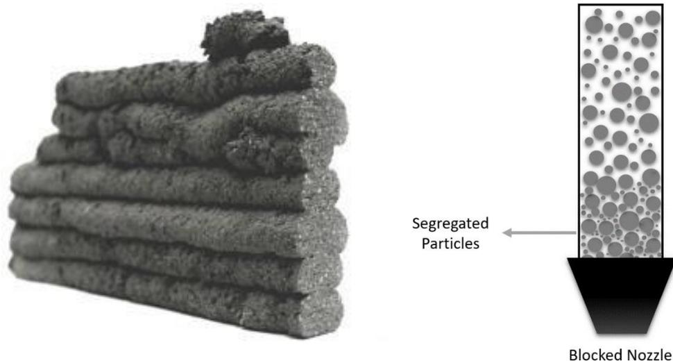
Figure 16: (Left) Layers Discontinuity and Surface Defects [120] (Right) Nozzle Blockage
