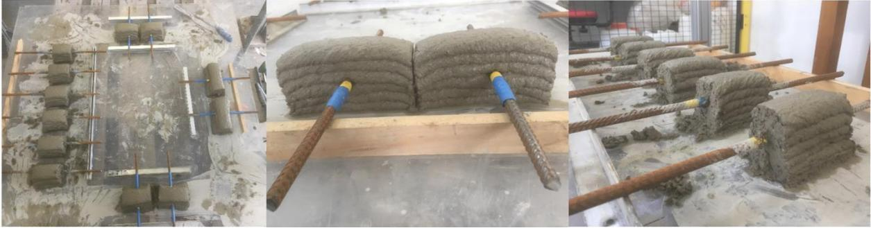
*Figure 5: Parallel and Perpendicular printed samples after being Cut*
