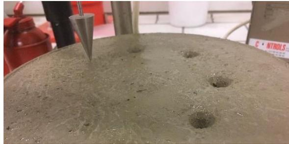
*Figure 2 Fall-Cone Test*
