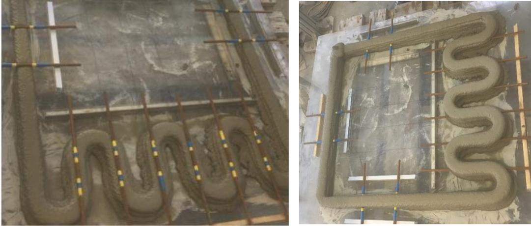
*Figure 4: 3D printed Pull-out samples*
