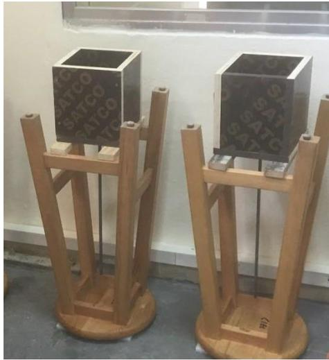
*Figure 2 Casting molds for Pull-Out samples*
