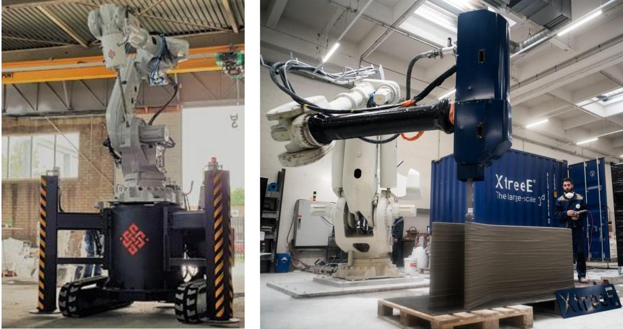
Figure 4: (Left) CyBe Construction (Right) XtreeE Printers [29]
