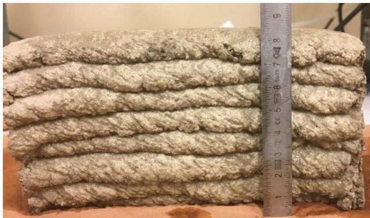
*Figure 3 Printed element using the Lab. Gun*
