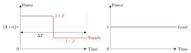
Figure 4.2: Input signals of the simulation with a single characteristic time-scale.
