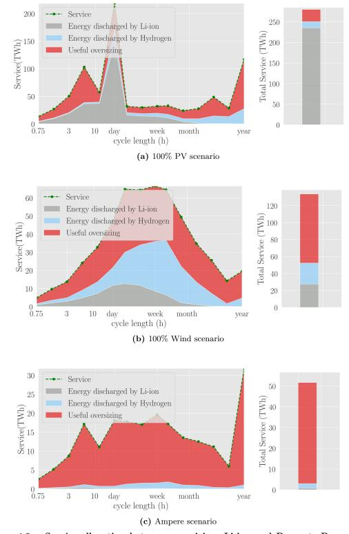
Figure 4.9: Service allocation between oversizing, Li-ion and Power-to-Power with hydrogen stored in steel bottles. Service is calculated for three different scenarios: 100 % PV (a), 100 % wind power (b) and the Ampère electricity generation mix (c) that includes 25 % of wind power and 10.5 % of photovoltaic. Left-hand figures depict Service decomposition over the 15 time-scales, right-hand figures the total Service, all time scales combined.
