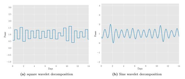
Figure A.2: 2013 PV power supply filtered with  $\Delta T = 24h$  square and sine wavelets.
