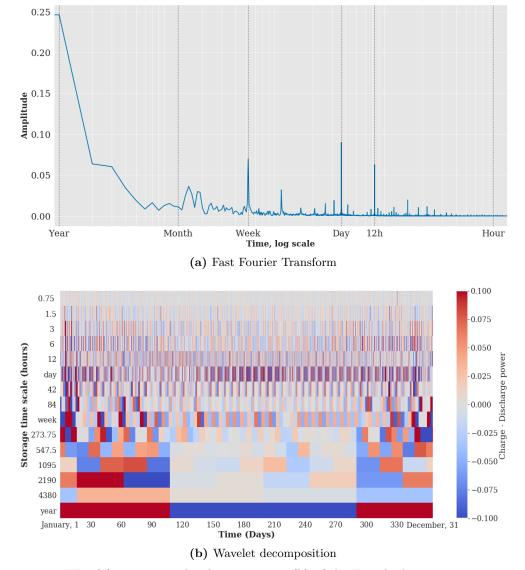
**Figure 3.4:** FFT (a) versus wavelet decomposition (b) of the French electricity consumption in 2018.
