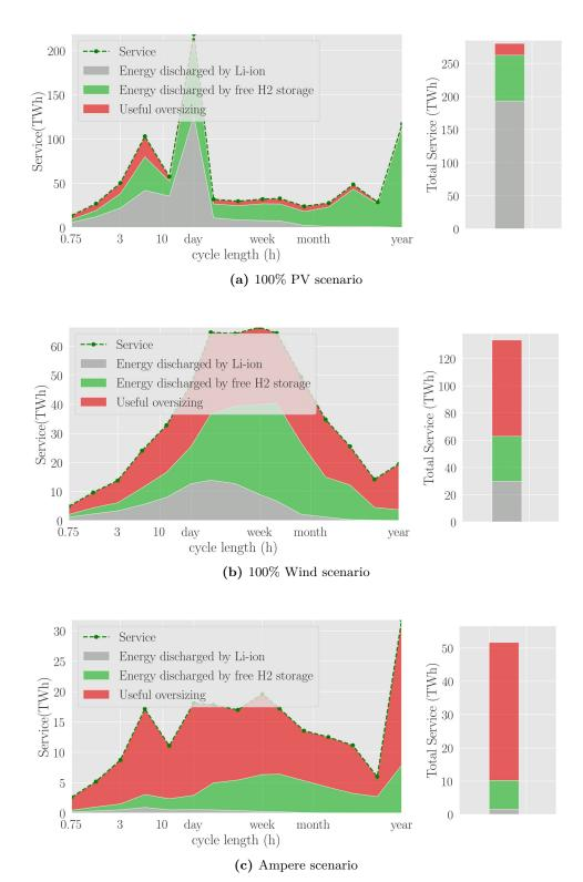
Figure 4.10: Service allocation between oversizing, Li-ion and Power-to-Power with hydrogen stored for free. Service calculated for three different scenarios: 100 % PV (a), 100 % wind power (b) and the Ampere electricity generation mix (c) that includes 25 % of wind power and 10.5 % of photovoltaic. Left-hand figures depict Service decomposition over the 15 time-scales, right-hand figures the total Service, all time scales combined.
