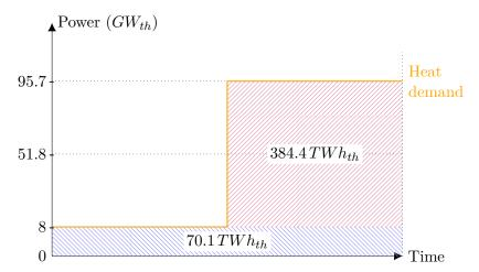
Figure 5.3: Amplitude of the heat demand signal. Values in the power axis are presented as an indication but are not to scale.
