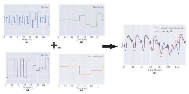
Figure 3.3: Illustration of the wavelet decomposition. Wavelet signals of time-scales  $\Delta T = 12$  hours (a), 1 day (b), week/4 (c) and week/2 (d) are summed and placed on top of the original signal (e). Shorter time scales are omitted here to show an imperfect approximation.
