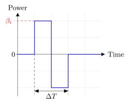
**Figure 3.6:** Square wavelet indexed by *i* in time, of time scale  $\Delta T$ . We refer to its amplitude by  $\beta_i$ .
