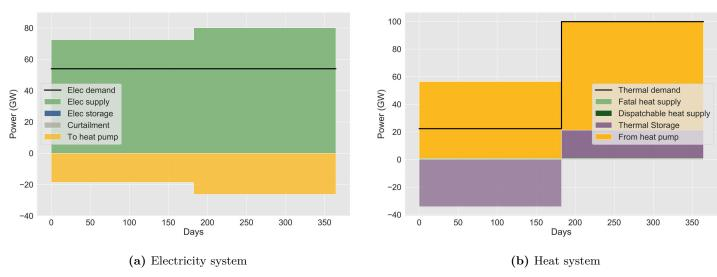
Figure 5.11: Behavior of electricity (a) and thermal (b) systems in the reference case.
