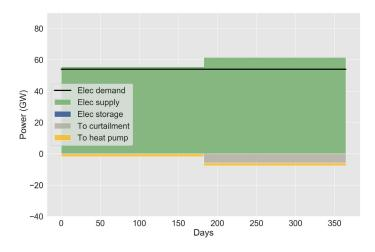
Figure 5.6: Electricity system operating modes: The production (green) is oversized. HPs are used with a constant power in both summer and winter to convert electricity into heat. The excess that remains is curtailed.
