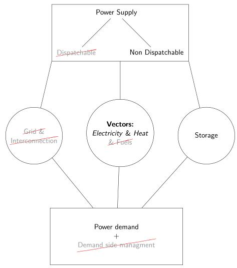
Figure 1.1: Sketch of the energy system considered and its boundaries. The flexibility solutions considered in this work will rely entirely on storage capacity and heat vector complementarity. Interconnections, demand-side management or dispatchable sources will not be considered.
