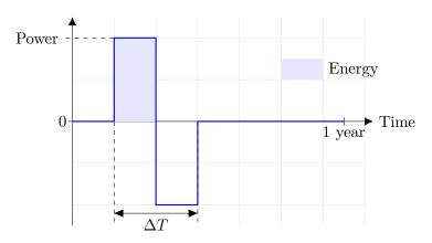
Figure 3.2: An example of a Haar wavelet with its three characteristics: *Energy, Power*, and charge-discharge duration  $time\text{-}scale\ \Delta T$ .
