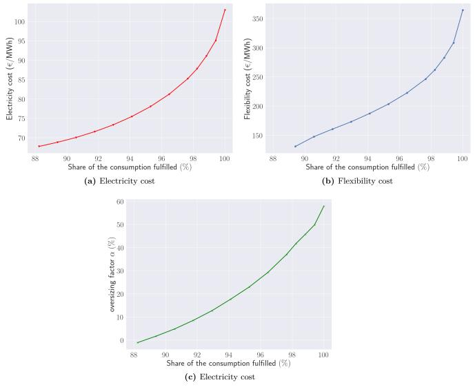
Figure 4.11: Sensitivity analysis for the Ampère scenario with Li-ion and  $H_2$  stored in bottles. Figure (a) shows the electricity cost as a function of the share of the electricity demand satisfied. With the same x-axis, (b) shows the cost of flexibility and (c) the oversizing factor  $\alpha$ .
