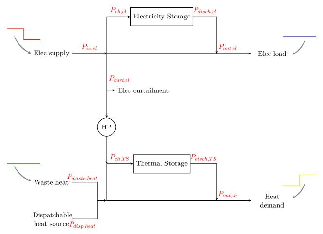
Figure 5.1: Representation of the energy system considered. Electricity and heat systems are coupled through a heat pump (HP).
