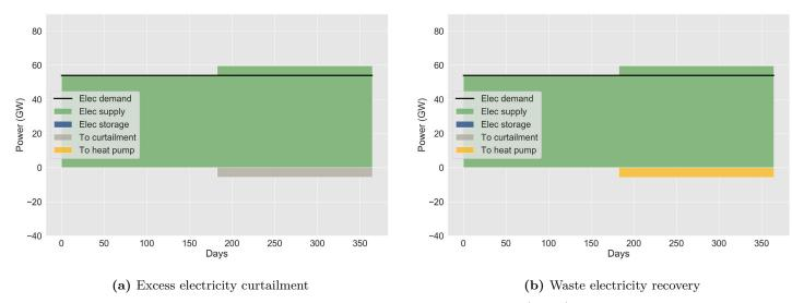
**Figure 5.4:** Electricity system operating modes: The production (*green*) is oversized so that its minumum value is equal is to the consumption (black line). In (a), excess electricity is curtailed (*gray*), in (b) the excess is converted into heat through the heat pump (*yellow*).
