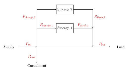
**Figure E.1:** Representation of the energy system. Electricity supply can either be directly consumed, stored or curtailed.
