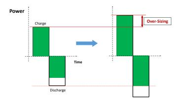
**Figure 3.10:** When the round trip efficiency  $\eta$  of a storage device is <1, the production has to be oversized by a factor  $\alpha$ . It enables to charge more energy in order to discharge as much as needed.
