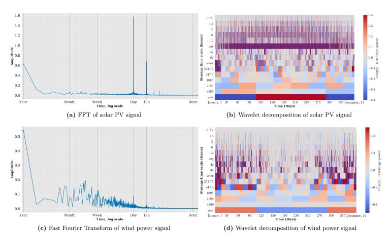
**Figure 3.5:** FFT (left) versus wavelet decomposition (right) of two French power generation signals in 2018: PV signals are at the top, wind power generation at the bottom.
