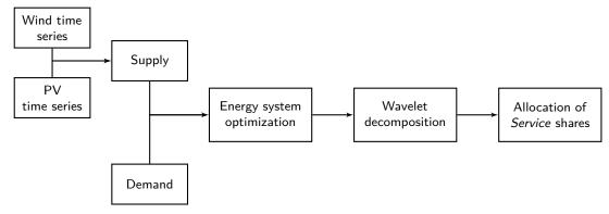
Figure 4.8: Description of the methodology in four steps of the simulation carried with real time series. First, the power generation signal is created. Second, with this input data, the energy system is optimized. Third, the output time series of the optimization are decomposed using the wavelet methodology. Finally, we analyzed which flexible mean provides the required Service that matches electricity demand and supply: storage 1, 2 or oversizing.
