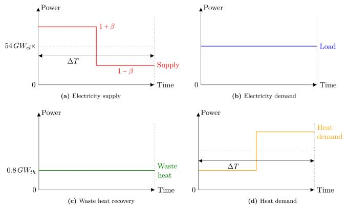
**Figure 5.2:** Input electricity (top) and heat (bottom) signals of the simulation with a single characteristic time-scale.
