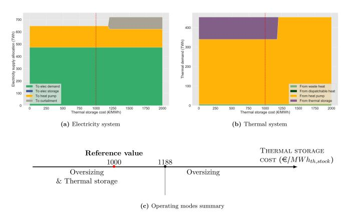
Figure 5.12: Thermal Storage cost sensitivity analysis.
