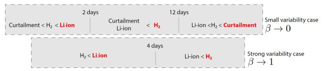
Figure 4.3: Calculation of  $\Delta T_{eq}$  between the use of Li-ion, hydrogen or oversizing. Those results corresponds to the framework "Single time-scale". It shows which is the most relevant technology to be used, depending of the time-scale usage. Warning note: the cost of the optimal technological solution does not appear. It skyrockets for long time-scales and strong variability.
