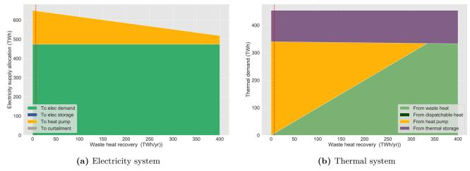
Figure 5.18: Waste heat recovery sensitivity analysis.
