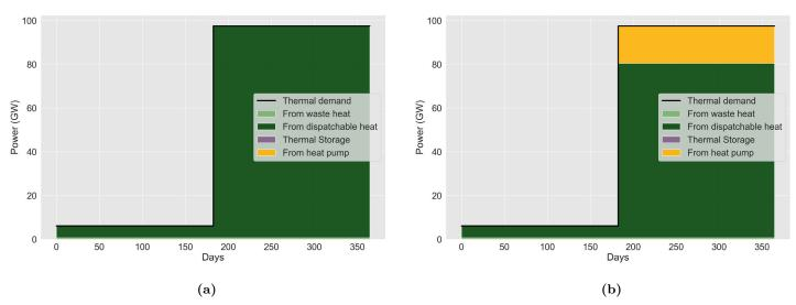
Figure 5.8: Thermal system operating modes: Heat boilers are both used in summer and winter. In (a), it is the unique heat source. In (b), heat is also provided by heat pumps in winter.
