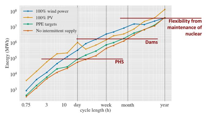
**Figure 3.9:** Zoom of Figure 3.7a. It shows the flexibility requirements in terms of energy capacity (y-axis) of 4 power generation scenarios, calculated for each time scale (x-axis), going from 45 minutes (left) to one year (right). The need for flexibility is compared to the French flexible means: PHS, hydroelectricity dams. We also add the flexibility provided by deliberate nuclear shutdowns for maintenance. More details on these flexible means are available in Table 3.1 and chapter 3.
