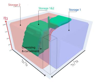
**Figure 4.5:** Mapping of the flexibility means used by the optimal solutions for the *small variability case*, depending on the relative costs of the storages, and storage 2 efficiency. The red area corresponds to storage 2, the blue to storage 1. Where the space is green, both storages are used in combination. Where there is no color, *Service* is entirely provided by the over-sizing.
