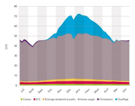
**Figure 2.7:** Source: [13]. 2015 French electricity consumption, power called per uses. The upper blue part is the electricity used for heating and it corresponds to 14 % of total electricity demand, i.e., 14 TWh in 2015. From bottom to top, we observe *cooking*, *domestic water heating*, *lighting*, *others*, *Air conditioning* and *heating*.
