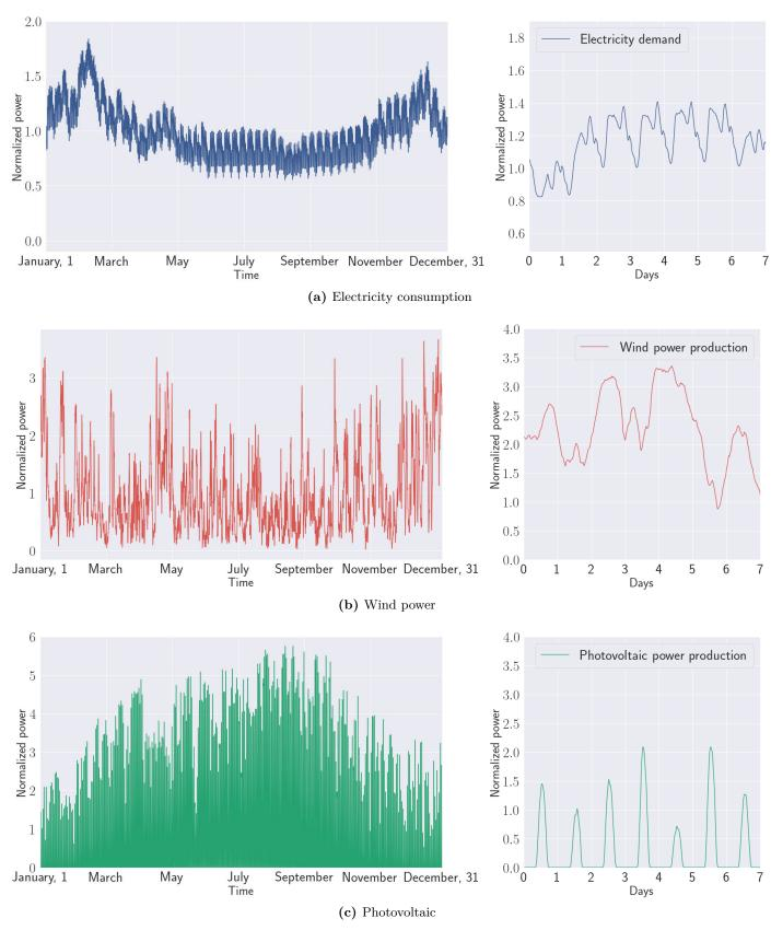
**Figure 2.6:** One year of electricity consumption in France (a), wind energy production (b) and photovoltaic production (c). All signals are normalized by their average power. Time-series correspond to the year 2012. The figures on the right are a zoom of the first week of the year.
