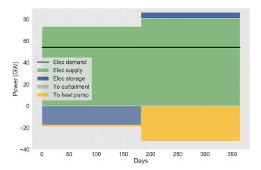
Figure 5.7: Electricity system operating modes: The production (*green*) is oversized. Excess electricity is: 1) charge in summer (*blue*) and discharged in winter, 2) converted into heat.
