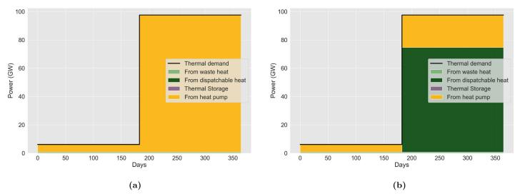
Figure 5.9: Thermal system operating modes: Heat pumps are used both in summer and winter. (a) shows a case where HPs entirely provide the required heat. In (b), the demand is also supplied with dispatchable heat in winter.
