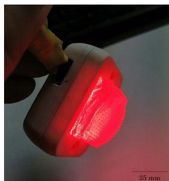
Figure 4.6 – Photo of the MN patch stuck to the LED array thanks to the double sticky layer realized with modified PDMS.
