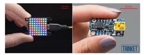
Figure 4.3 – Left: Light emitting system chosen: Adafruit Dotstar High Density  $8 \times 8$  grid. Right: Arduino microcontroller: Adafruit Trinket.
