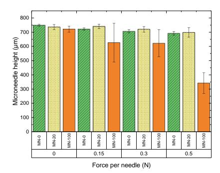
Figure 2.7 – Mechanical behaviour of  $MN_t$  after compression at different forces. Analyses were performed on three different patches with at least 10 height measurements on different microneedles from each patch. Results are presented as mean  $\pm$  standard deviation.
