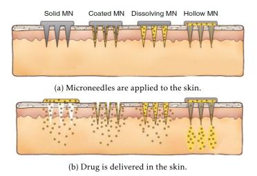
Figure 1.7 – Methods of drug delivery to the skin using different kind of microneedles [86]
