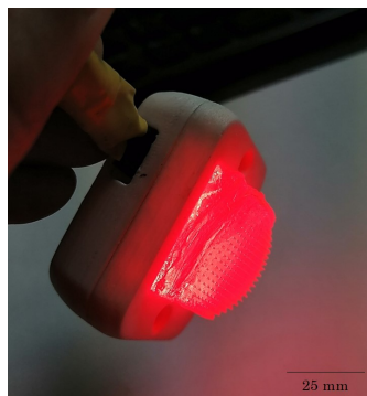
Figure 4.6 – Photo of the MN patch stuck to the LED array thanks to the double sticky layer realized with modified PDMS.
