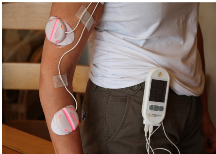
Figure 4.2 – Portable light emitting system Ambulight® used for PDT treatment.
