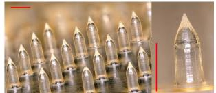
Figure 1: Digital microscopy images of MN-patch fabricated by solvent casting molding method. (Left:  $MN_l$ -0, right:  $MN_t$ -20.) Scale bars represent 500  $\mu$ m.
