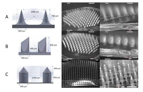
Figure 2.4 – Different shapes of HA-based microneedles (HA concentration : 5% w/w). A: Conical microneedles included in a circle shaped patch (MN number : 163. Patch surface:  $2.54\,\mathrm{cm}^2$ ). B: Beveled microneedles included on a circle shaped patch (MN number: 138. Patch surface:  $2.54\,\mathrm{cm}^2$ ). C: "Pencil-tip" shape microneedles included on a squared shaped patch (MN number: 400. Patch surface:  $20\times20\mathrm{cm}^2$ ).
