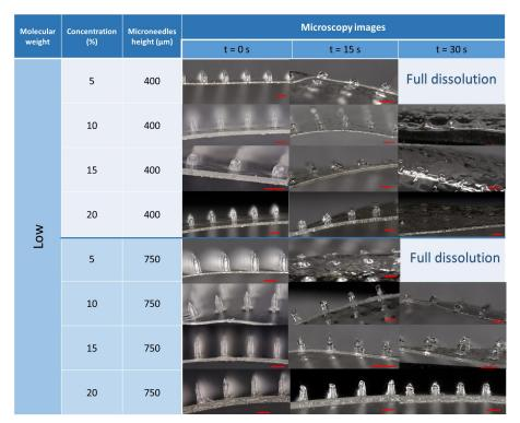
(a) Representative microscopic images of low HA  $((5.50\pm0.04)\times10^4~{\rm g~mol}^{-1})$  at different concentrations: 5%, 10%, 15%, and 20% (w/v) before application on the skin phantom (0 s) and after 15 s or 30 s dissolution in phantom skin. Two MN heights were also investigated.
