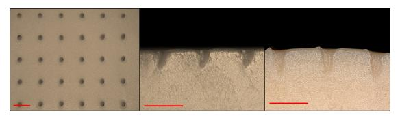
Figure 10: Left: top view observation of phantom skin after MN-patch removal. Middle: cross section of phantom skin after  $MN_l$  removal. Right: cross section of phantom skin after  $MN_l$  removal. Experiments repeated 5 times. Scale bars represent  $1000 \, \mu \text{m}$ .
