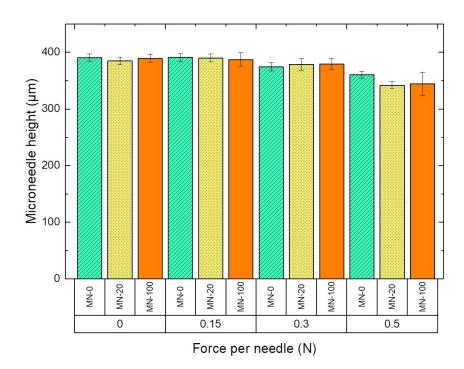
Figure 8: Mechanical behaviour of  $MN_l$  after compression at different forces. Analyses were performed on three different patches with at least 10 height measurements on different microneedles from each patch. Results are presented as mean value  $\pm$  standard deviation.
