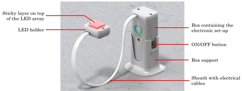
(a) Schematic representation of the embedded light device.
