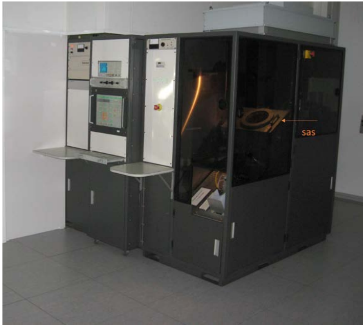
Fig. 3.4: Photography of the implanter at LAAS in Toulouse. The beam comes from the left side and arrives on the sample located in the chamber on the right.
