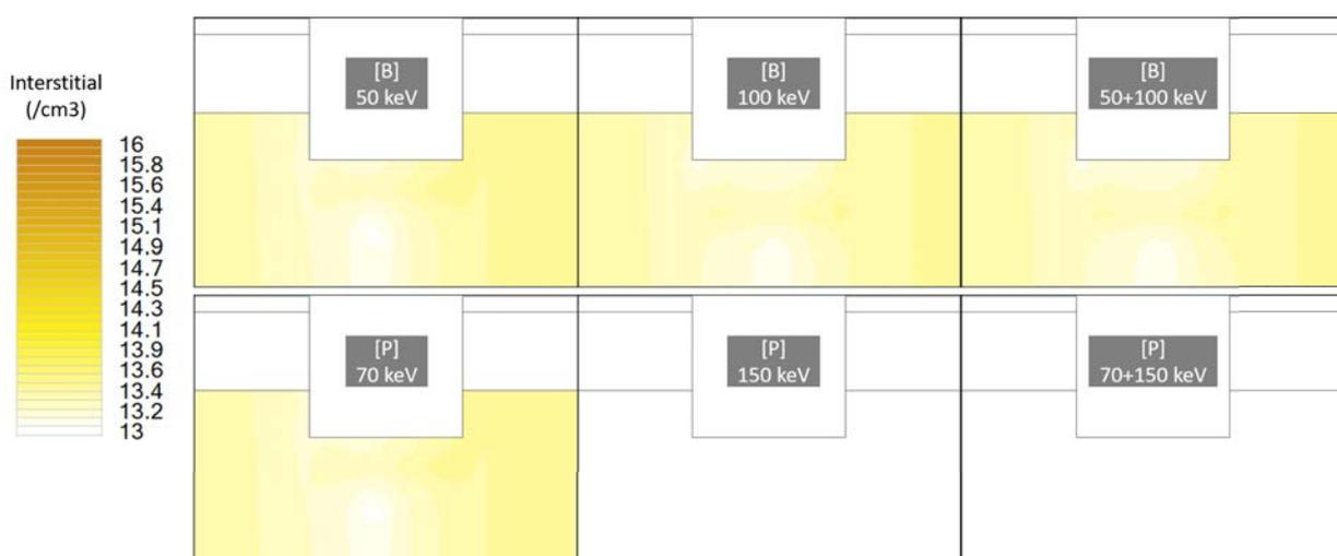
Fig. 5.19: Interstitial defects simulations on separated Boron (top) and Phosphorus (bottom) implantations for an annealing of 300 s at 950 °C.
