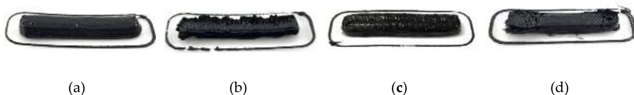
Figure 5-16 Samples printed with STT tip under 4 configurations: (a) without magnetophoresis; and with magnetophoresis consisting of (b) vertical array; (c) horizontal array; and (d) Halbach array
