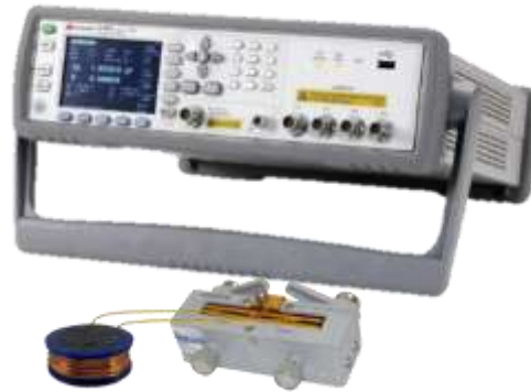
Figure 2-7 Photo of LCR Meter (Keysight E4980AL, Agilent)
