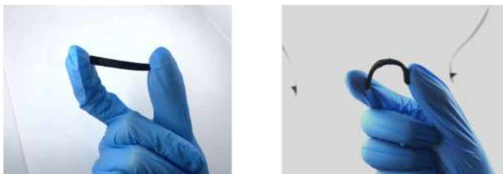
Figure 4-23. Flexible ferromagnetic composite based PDMS polymer elaborated with 30% \text{Fe}_3\text{O}_4 particles
