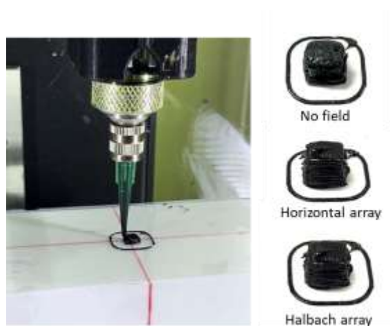
Figure 5-17 Cubic-shape samples printed under the two types of horizontal magnetic field.
