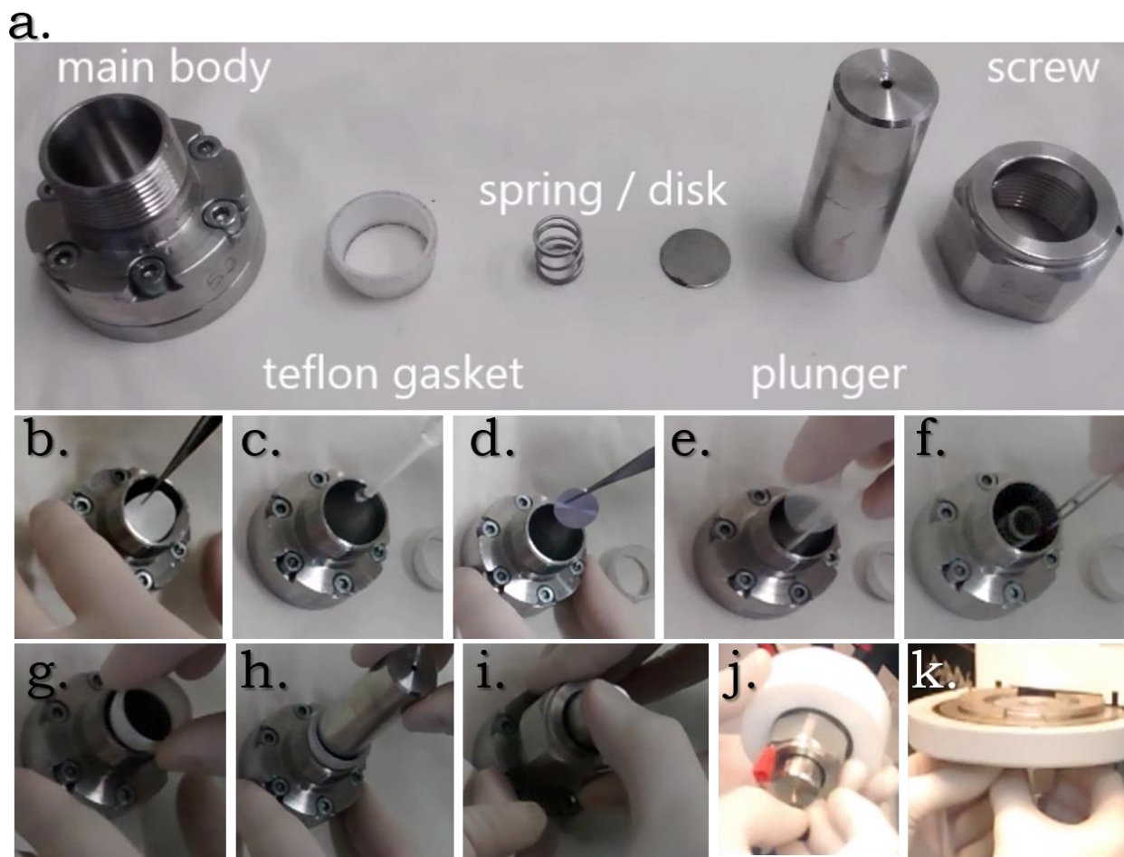
Figure 2.4. a. Different parts of the cell. Operando cell assembly: after the active material is placed, the b. and c. the separator with electrolyte, d. the stainless-steel with spread Li metal. e. acetate film to isolate. f. and g. spring and Teflon gasket, respectively, and h. the plunger is placed. i. The screw is turned, applying pressure to close the cell. j. the cell is connected to a potentiostat-galvanostat, and k. the cell is placed on the diffractometer holder. Adapted from [10].
