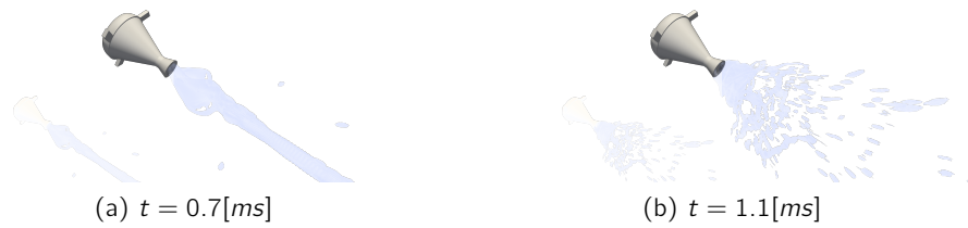
Figure 5.22 – Contour plot of the iso-surface defined by liquid volume fraction \alpha_l = 0.3 of the Silvercrest primary injector. Startup phase on the mesh C. On the bottom left we can see the shadow of the liquid volume fraction .
