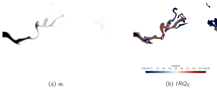
Figure B.1 – On the left: liquid volume fraction surface plot of a snapshot of the box configuration defined along the thesis. \alpha_l = 0 to 1 . On the right: IRQ_{\Sigma} surface plot, on the clipped field of liquid volume fraction \alpha_l \in [0.1, 1] .
