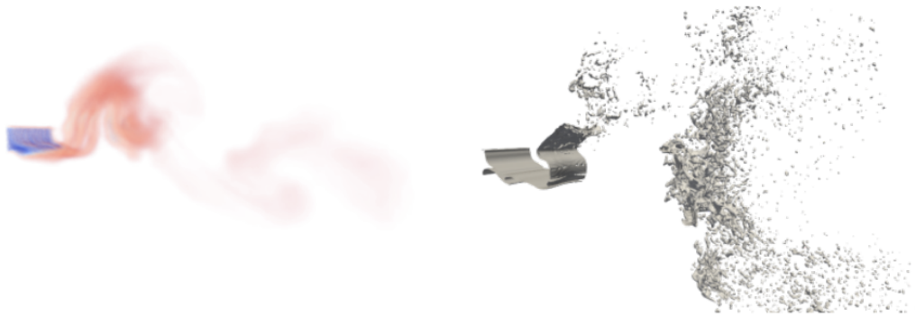
Figure 3.8 – Instantaneous picture of the flapping liquid sheet. On the left CEDRE(HR) simulation. The colorscale goes from low levels of \alpha_l (blue) to high levels (red). On the right ARCHER simulation. The iso-contour represents the 0 iso-value of the level-set distance function .
