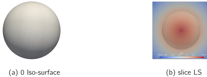
Figure A.1 – Domain of computation for the test of the curvature algorithm on a sphere. On the left the 0 iso-surface of the level-set function, on the right a slice of the field with the shadow of the level-set distance function 0 iso-surface.
