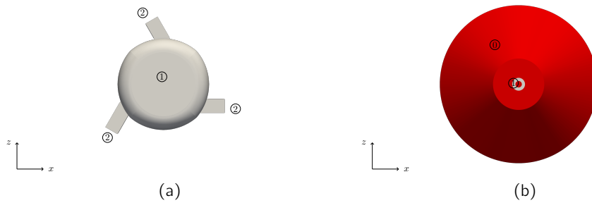
Figure 5.20 – Top view of the computational domain, marked with number to define the different boundary patch. On the left: top view of the primary injector. ② : inlet, ① : wall of the primary injector. On the right: top view of the external domain simulating the external environment. ① : air, ① : wall near the outlet of the injector.
