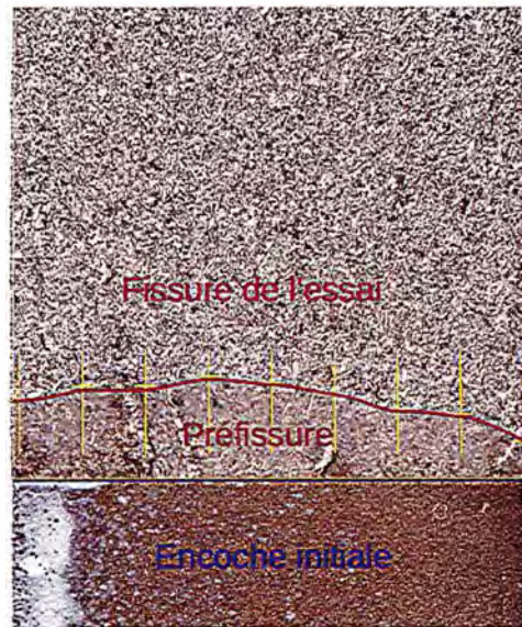
FIGURE 4.6 – Faciès de rupture
