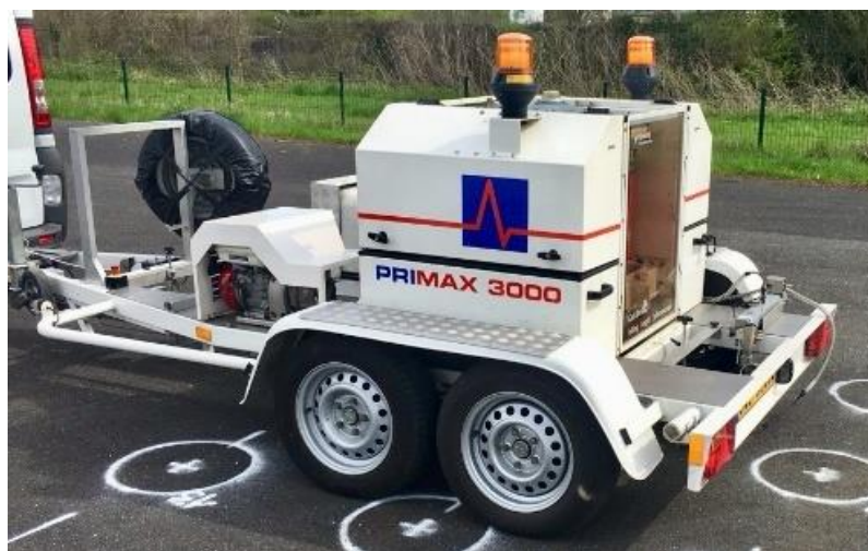
Figure 2.1 – HWD Carl Bro PRI3000 du STAC (photographie JM Roussel)
