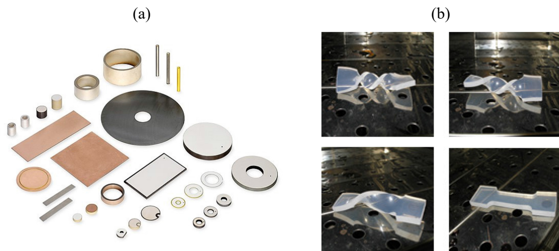
Figure 1.3 Examples of Smart Materials: (a) Piezoelectric and (b) Shape memory polymers (reproduced from Butaud et al. (2016)).
