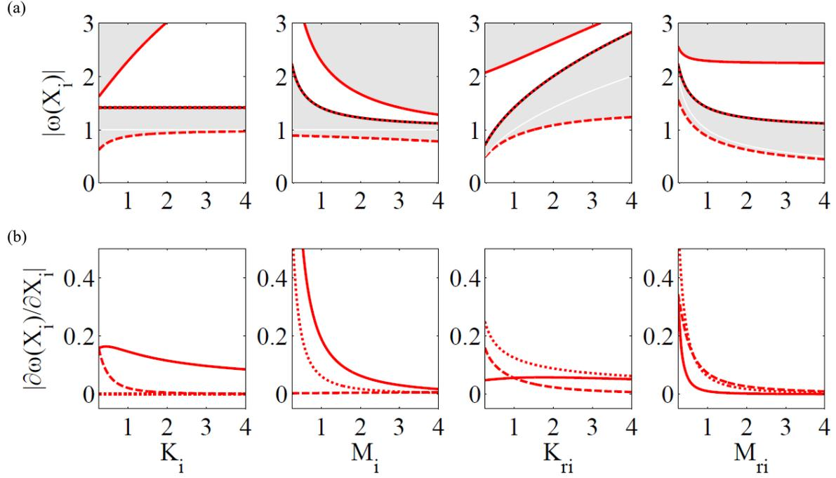
**Figure 2.9** (a) Parametric variation of unit cell parameters on abscissa and frequency on ordinate for band gap envelopes (  $\square$  ), anti-resonance inside attenuation zone (  $\blacksquare$  ) and natural frequency (  $\dots$  ); band gap borders 1 (  $---$  ), 2 (  $\cdots$  ) and 3 (  $---$  ) and (b) their corresponding analytical derivatives for case 5.
