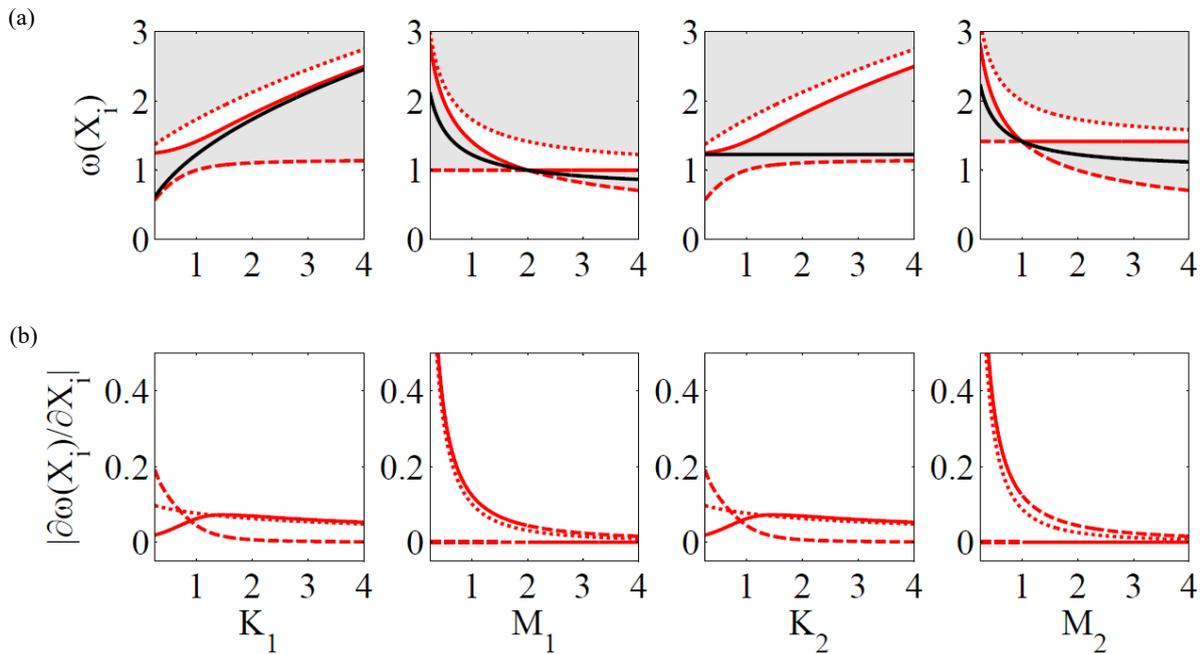
**Figure 2.8** (a) Parametric variation of unit cell parameters on abscissa and frequency on ordinate for band gap envelopes (■), natural frequency inside attenuation zone (—), band gap borders 1 (---), 2 (—) and 3 (····) and (b) their corresponding analytical derivatives for case 2.
