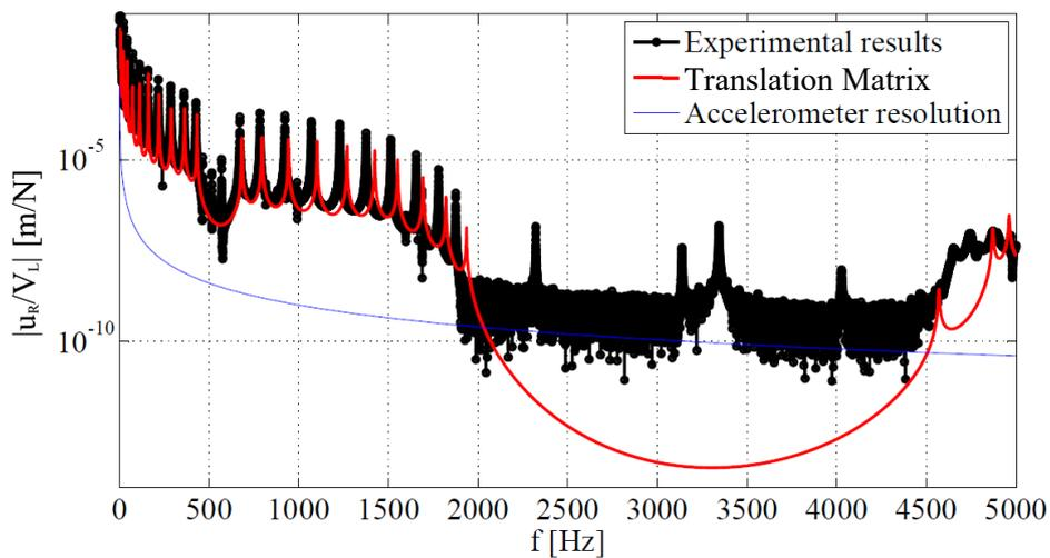
**Figure 4.5** Frequency response function obtained experimentally for a free-free periodic beam with 10 stepped unit cells.
