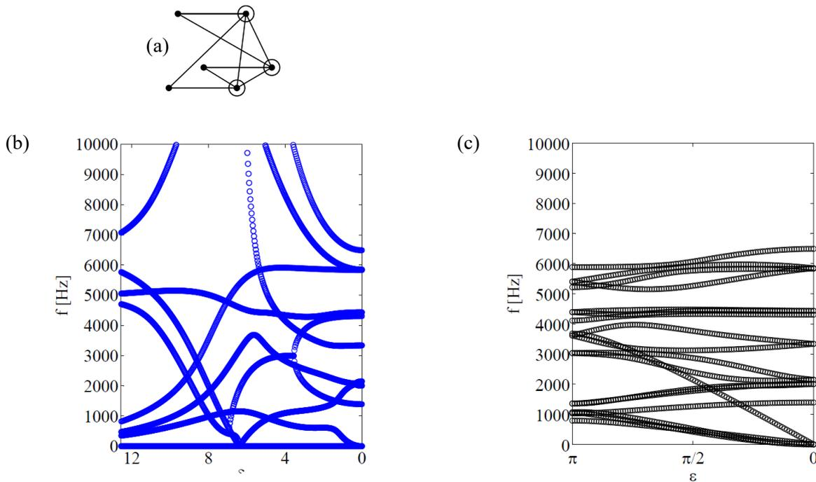
Figure 5.3 (b) Attenuation and (c) phase constants of truss unit cell (a) with concentrated mass on nodes.
