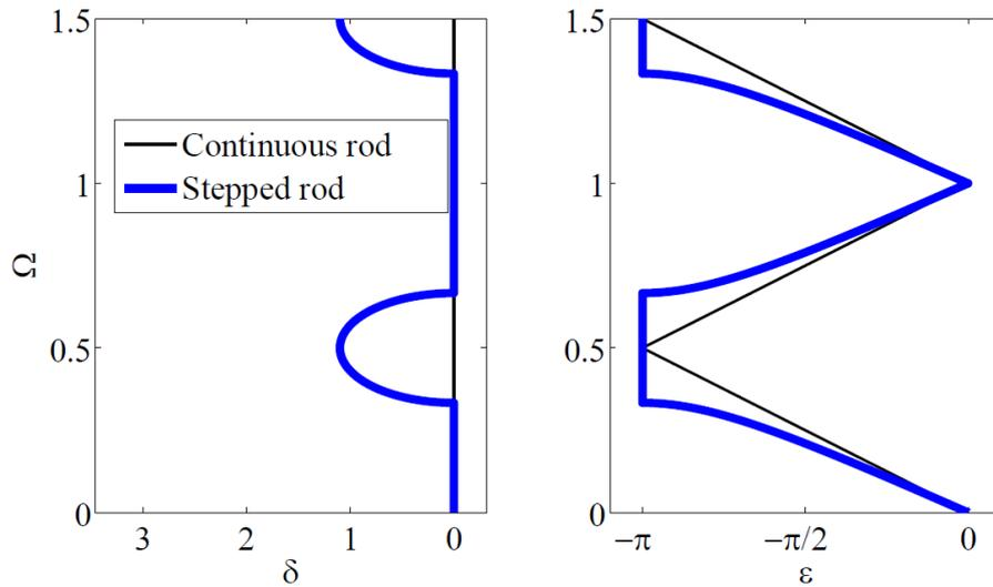
Figure 2.5 Dispersion diagram for a continuous rod and for a stepped rod.
