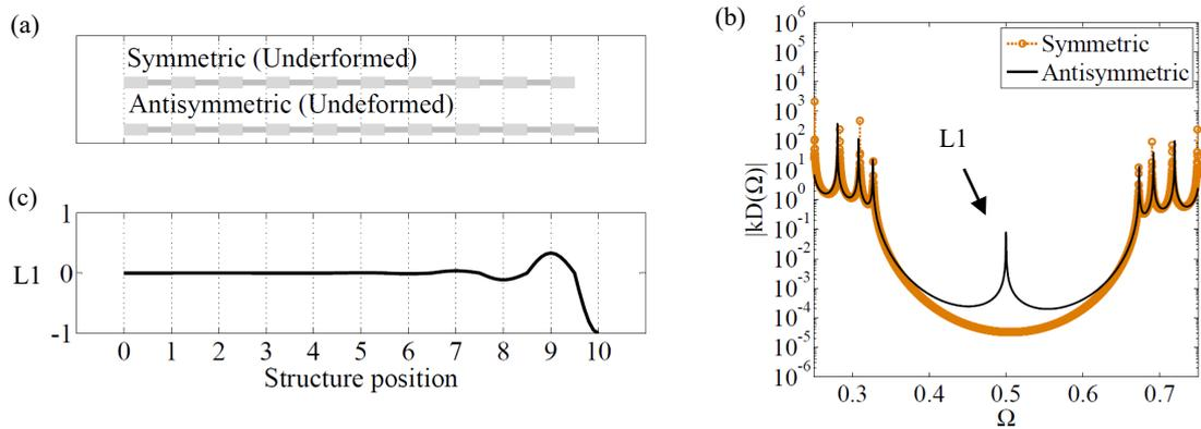
**Figure 2.14** Comparison between (a) symmetrical and antisymmetrical structures, their (b) FRFs and (c) the shape of localized mode L1 for antisymmetrical one.
