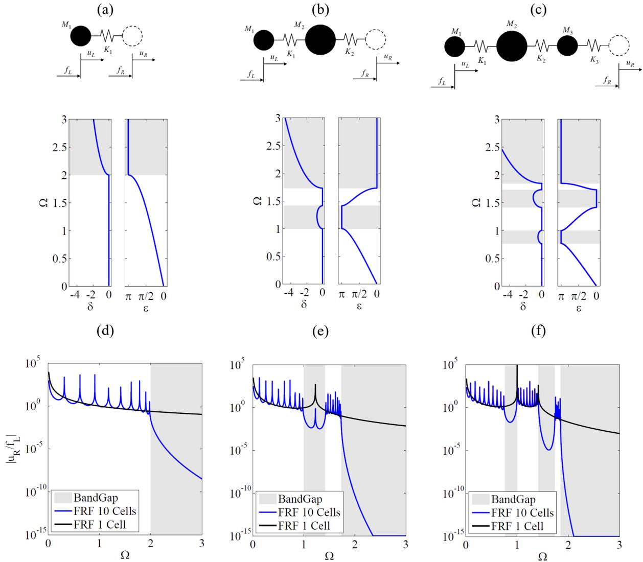
**Figure 2.2** Dispersion diagrams for different unit cells: (a) case 1, (b) case 2 and (c) case 3, and FRF amplitudes computed for 1 and 10 cells: (d) case 1; (e) case 2; (f) case 3.
