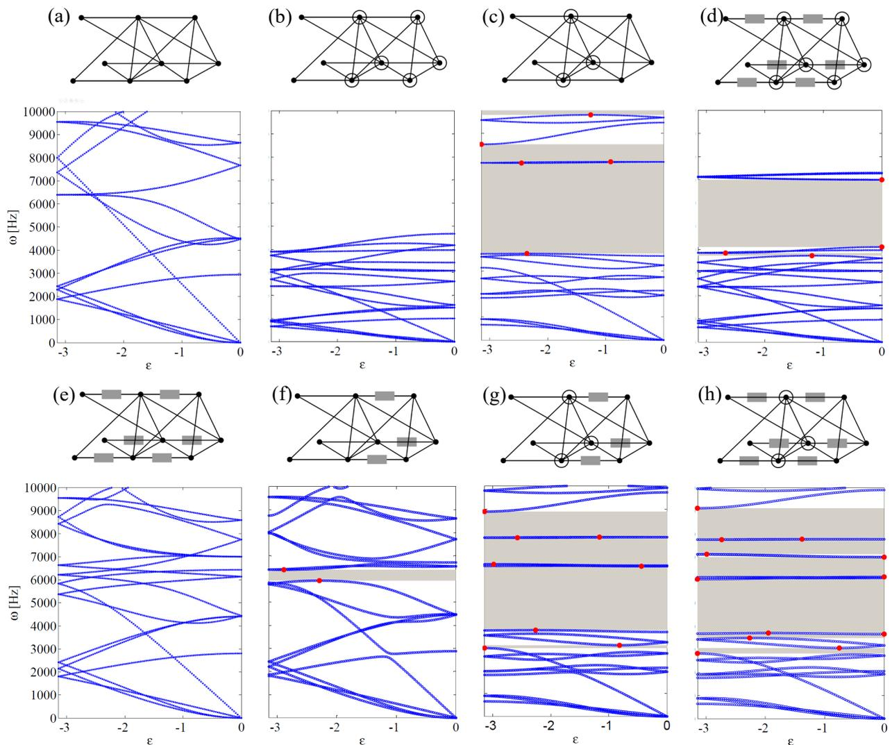
**Figure 5.5** Considered unit cells (a), (b), (c), (d), (e), (f), (g) and (h) with their respective dispersion diagrams.
