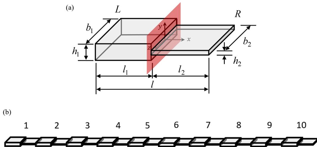
Figure 3.6 (a) Asymmetric beam unit cell and (b) its finite structure with 10 cells.
