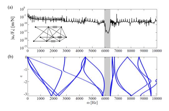
Figure 5.10 Band gap for (a) finite and (b) infinite structures considering the local resonance effect.
