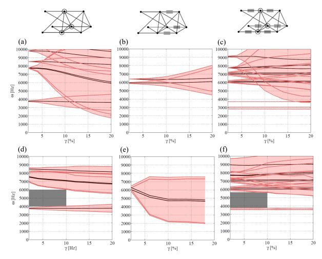
Figure 5.8 Bandgap bounds envelopes relatives to scenarios on Figures 5.3(c), 5.3(f) and 5.3(h), with: (a) mass as RV, (b) and (c) inductance as RV considering an infinite model (1 RV) with their corresponding (d), (e) and (f) for finite results with 10 RV.
