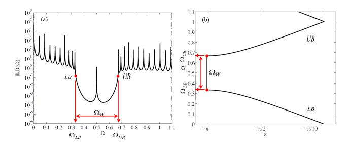
Figure 2.11 Bandgap borders for: (a) finite model and (b) infinite model.
