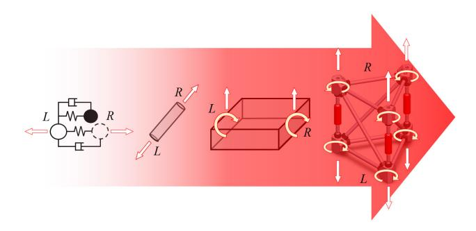
$\textbf{Figure 1.4} \ \text{Evolution from spring-mass systems, rods and beams to smart trusses.}$
