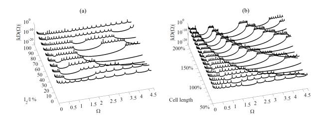
Figure 3.8 FRFs of stepped beam for several values of (a) discontinuity location and (b) cell length l.
