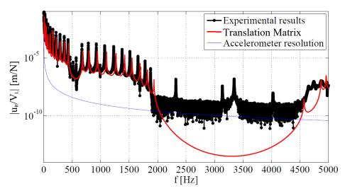
Figure 4.5 Frequency response function obtained experimentally for a free-free periodic beam with 10 stepped unit cells.
