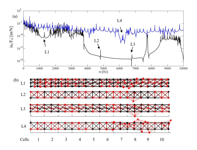
Figure 5.7 (a) FRFs with localization phenomena L1, L2, L3 and L4 and (b) their corresponding mode shape.
