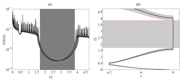
Figure 3.12 Robust bandgap for a stepped beam example considering (a) finite and (b) infinite structure.
