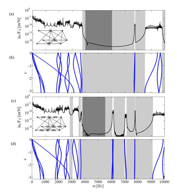
Figure 5.9 Robust band gaps for finite structures composed of 10 unit cells (a) and (c) and their respective dispersions diagramas for infinite structures (b) and (d).
