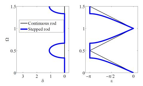
Figure 2.5 Dispersion diagram for a contrinuous rod and for a stepped rod.
