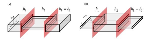
Figure 3.13 Symmetric unit cells (a) 1 and (b) 2 for flexural beams.
