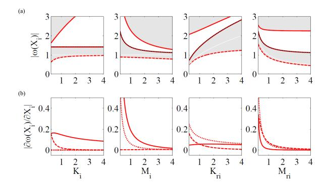
Figure 2.9 (a) Parametric variation of unit cell parameters on abscissa and frequency on ordinate for band gap envelopes ( ), anti-resonance inside attenuation zone ( ) and natural frequency ( ); band gap borders 1 ( -- ), 2 ( ·····) and 3 ( -- ) and (b) their corresponding analytical derivatives for case 5.
