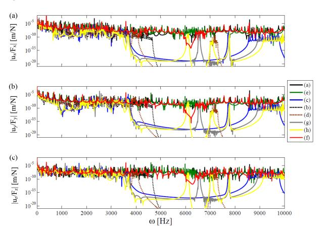
Figure 5.6 (a), (b) and (c) frequency responses of 8 scenarios periodic finite structures with 10 cells by exciting the firt node on direction x, y and z and observeing the corresponding dofs on the last unit cell.
