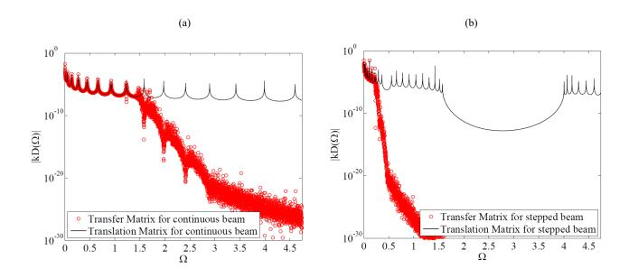
Figure 3.3 FRF Transfer Matrix method stability problem for: (a) continuous beam and (b) stepped periodic beam.
