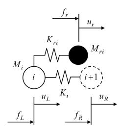
Figure 2.1 Example of spring-mass unit cell.
