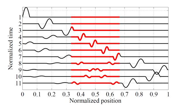
Figure 1.1 Wave propagating in a string with two density mismatches, in normalized positions 0.333 and 0.666, and fixed-fixed boundary contitions.
