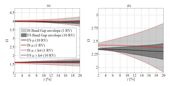
Figure 3.11 Confidence intervals for (a) LB, UB and (b) W for infinite structure (IS) with a stepped beam unit cell and for a finite structure (FS) with 10 stepped beam unit cells.
