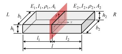
Figure 3.1 Representation of two continuous parts unit cell for a periodic beam structure.
