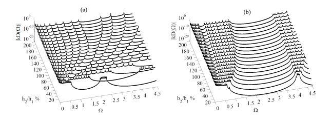
Figure 3.7 FRFs of stepped beam for several values of beam (a) thickness h<sub>2</sub> and (b) width b<sub>2</sub>.
