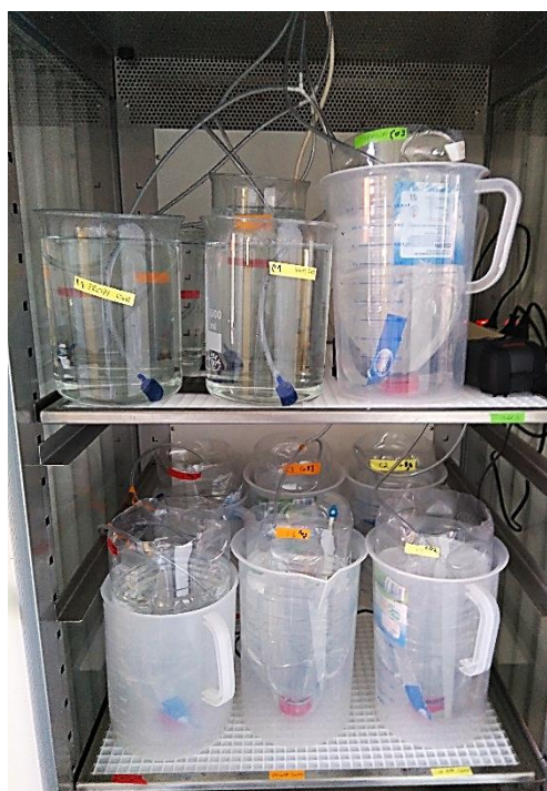
Figure 17 Glass or plastic three-liter beakers (depending on the hydrophobicity of the studied compound in the solution) used for the exposure of oyster larvae to pesticides in high yield. One beaker contains 500,000 larvae released by one mature oyster couple. The beakers are constantly oxygenated using aquarium airstones and kept in dark (due to the fast photodegradation of imidacloprid) in an incubator to maintain a constant temperature of 24 °C. (Original image by the author of the dissertation).
