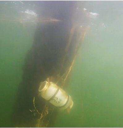
**Figure 22** Deployment of the caging devices by sailor Stéphane Bujan. Four devices were attached to each of the three buoys
