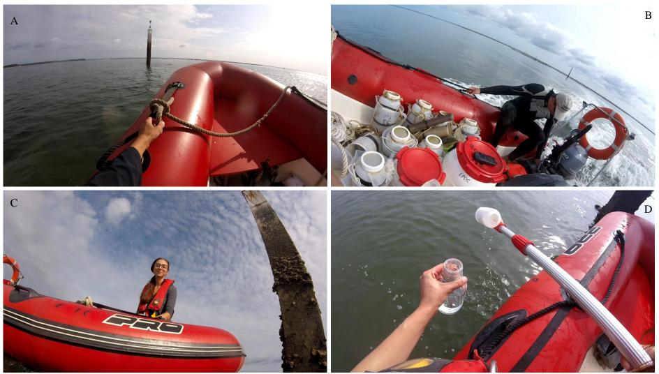
**Figure 21** Images illustrating the field work in Arcachon Bay. **A** Arrival to one of the selected buoys; **B** Boat filled with the devices full of water and larvae being transported to the laboratory at the end of exposure to be analyzed; **C** Preparation of devices to the sailor to attach them at the buoy; **D** Water sampling for the chemical analysis of pesticides
