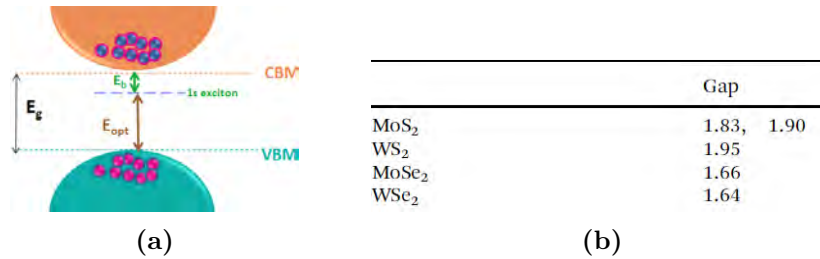
Figure 1.14: (a) Illustration of optical and electronic band-gap. (b) Optical band gap values for group VI TMDCs. Adapted from [28]
