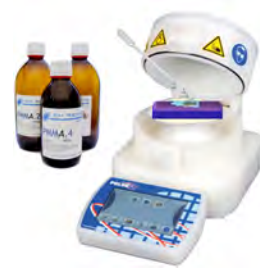
Figure 3.5: The resist spinner system. The wafer is maintained onto a chuck with vacuum. The resist is dispensed at the center of the wafer just before spinning.
