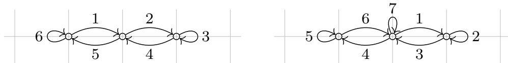
Figure 4.3: Minimal example showing the starting point has an impact on the solution. On the left, the starting point is the leftmost city, while on the right, the starting point is the middle city.
