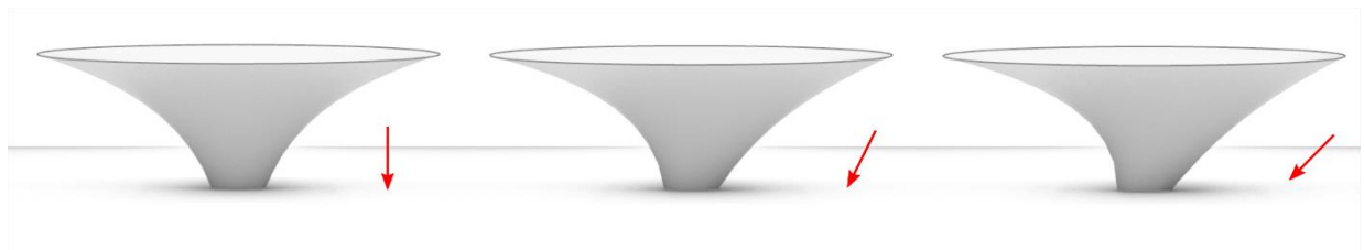
Figure 6.44: i-minimal membranes constructed on the same boundary, but with different isotropic directions
