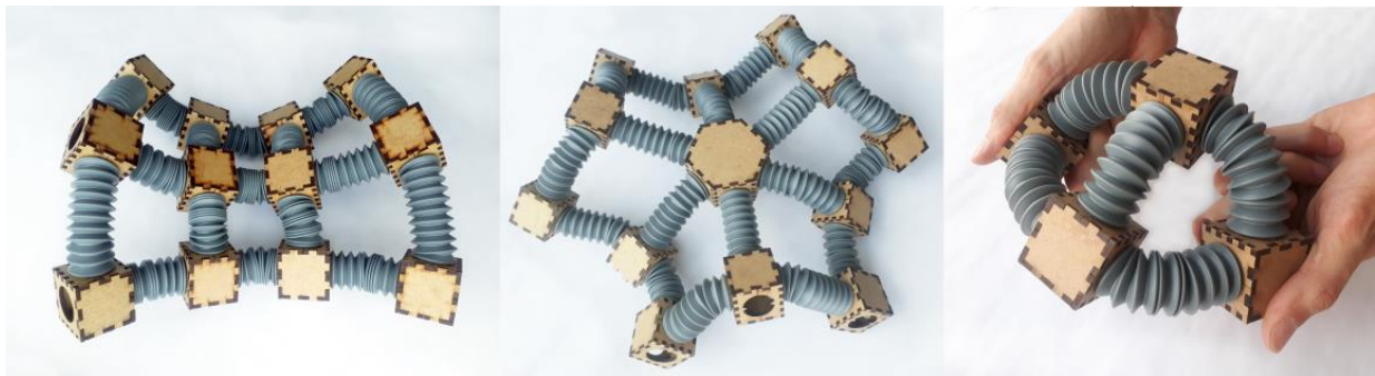
Figure 7.1: Mockups that replicates the behavior of a curvature line network through mechanical constraints. Left: Without umbilics. Middle: Umbilic of index -1/2 . Right: Umbilic of index +1/2
