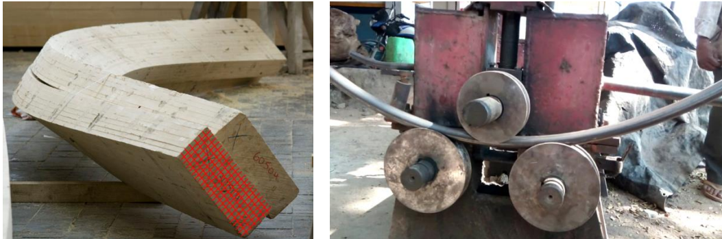
Figure 3.1: Left: A nonplanar gluelam beam (Courtesy of Design-To-Production (Zürich)) Right: Cold-bending of a steel profile (©Mallela Gbrs)
