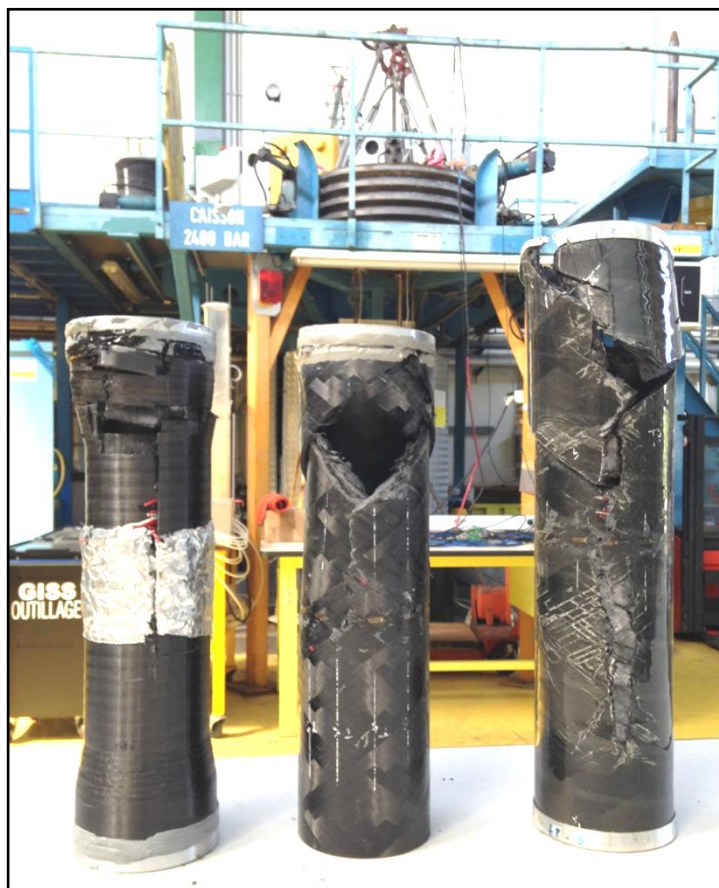
Figure 125 : Cylinders after implosion (left) C/PA6 [0/±88] (middle) C/PA6 [±55] (right) C/Epoxy [±55]
