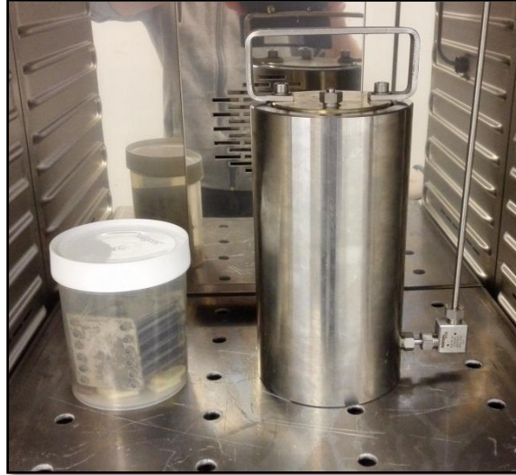
Figure 20 : (Left) 1 bar reference (Right) Test performed at 500 bar inside 40°C oven
