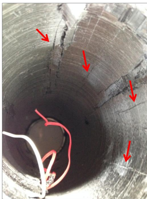
Figure 128 : Kinkbanding failure observed inside the [0/±88] cylinder
