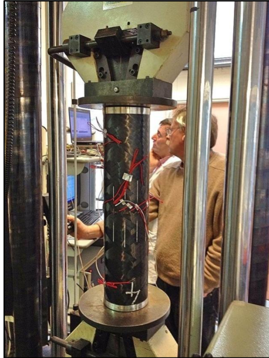
Figure 25: Axial compression test
