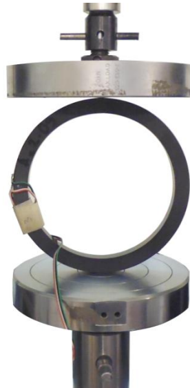
Figure 26: Radial compression test
