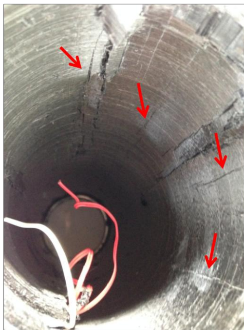
Figure 128 : Kinkbanding failure observed inside the [0/\pm 88] cylinder
