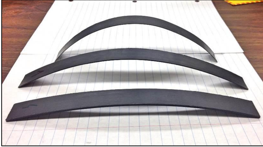
Figure 32 : Asymmetric laminates, from back to front: [0_2/90_2] , [0_4/90_4] and [0_8/90_8]
