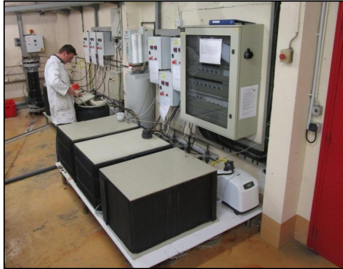
Figure 19 : Sea water aging tanks at Ifremer
