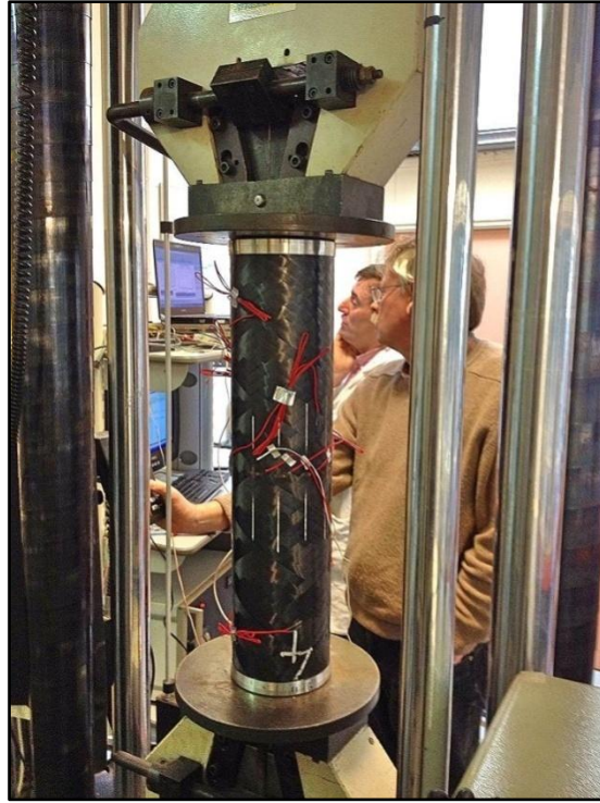
Figure 25: Axial compression test
