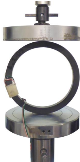
Figure 26: Radial compression test
