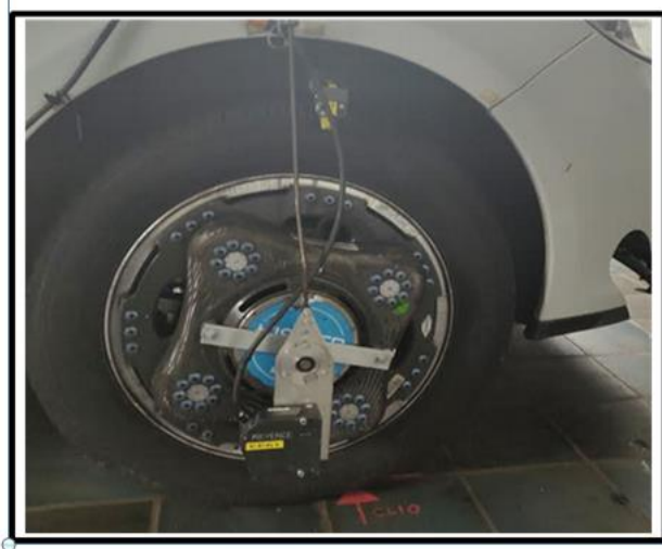
Figure 91 Dynamometric wheel mounted on the front right tyre
