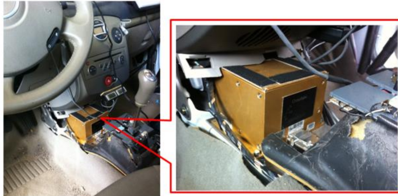
Figure 87 Inertial unit position
