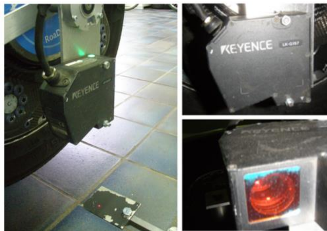
Figure 94 Tyre deformation sensor
