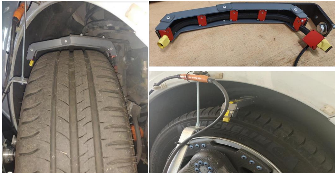
Figure 93 MB Flex infrared sensor for multi-beam flexible system
