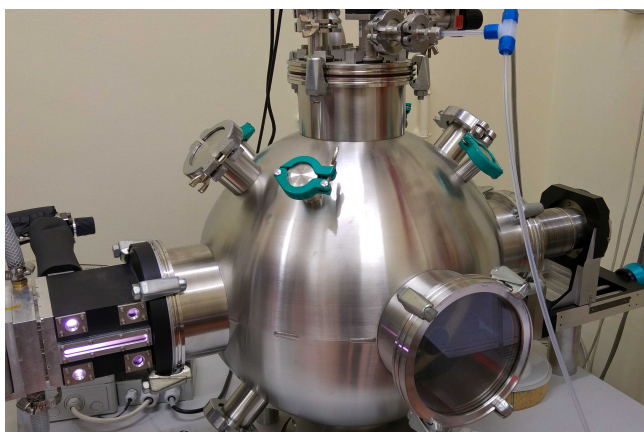
Figure 1.13: Photography of the BUBBLE vacuum setup with PEGASES running on argon, and setup adapted for Langmuir probe measurements.
