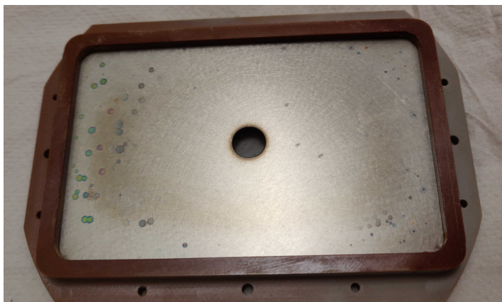
(a) Grid 1, used during the optical diagnostics. There is only one hole. The center hole is 1 cm in diameter.
