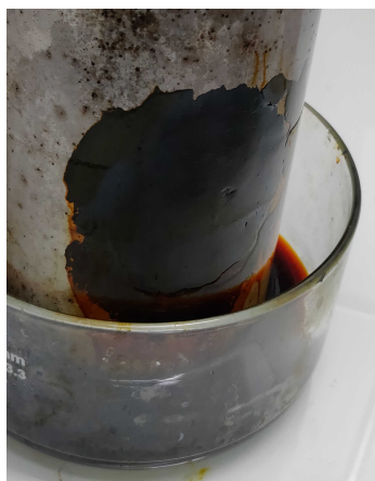
Figure 1.17: A layer of I_2 remaining on the liquid N_2 trap during a cleaning process. It is removed with ethanol. Using the wash bottle as some kind of pressure washing machine does really help.
