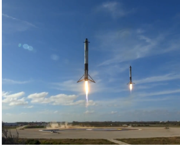
Figure 1.4: Two Falcon Heavy boosters from SpaceX landing after deploying its second stage. Credits: SpaceX.
