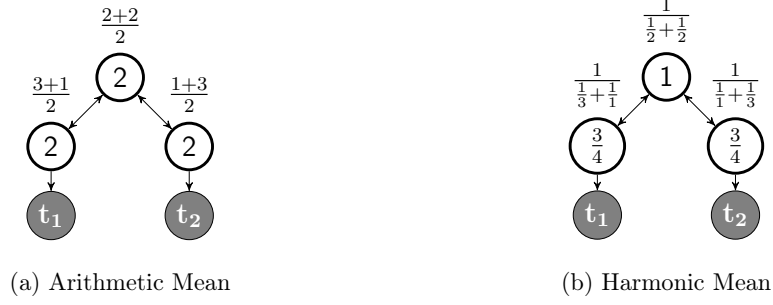
Figure 3.2: Difference between node distance defined in terms of arithmetic mean versus harmonic mean. Node distance is shown in the white circles. The targets are marked in gray [BPNR17].
