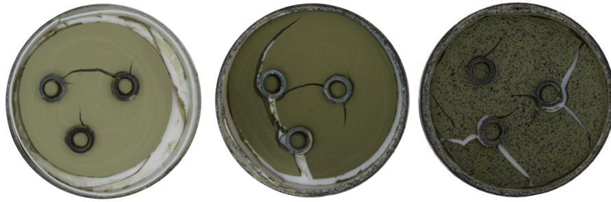
Figure 4.11 – Different crack patterns are observed on similar configurations.
