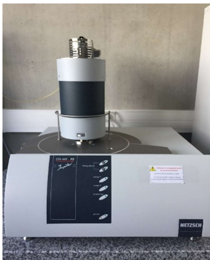
Fig. 3.15. Thermal analyzer device.
