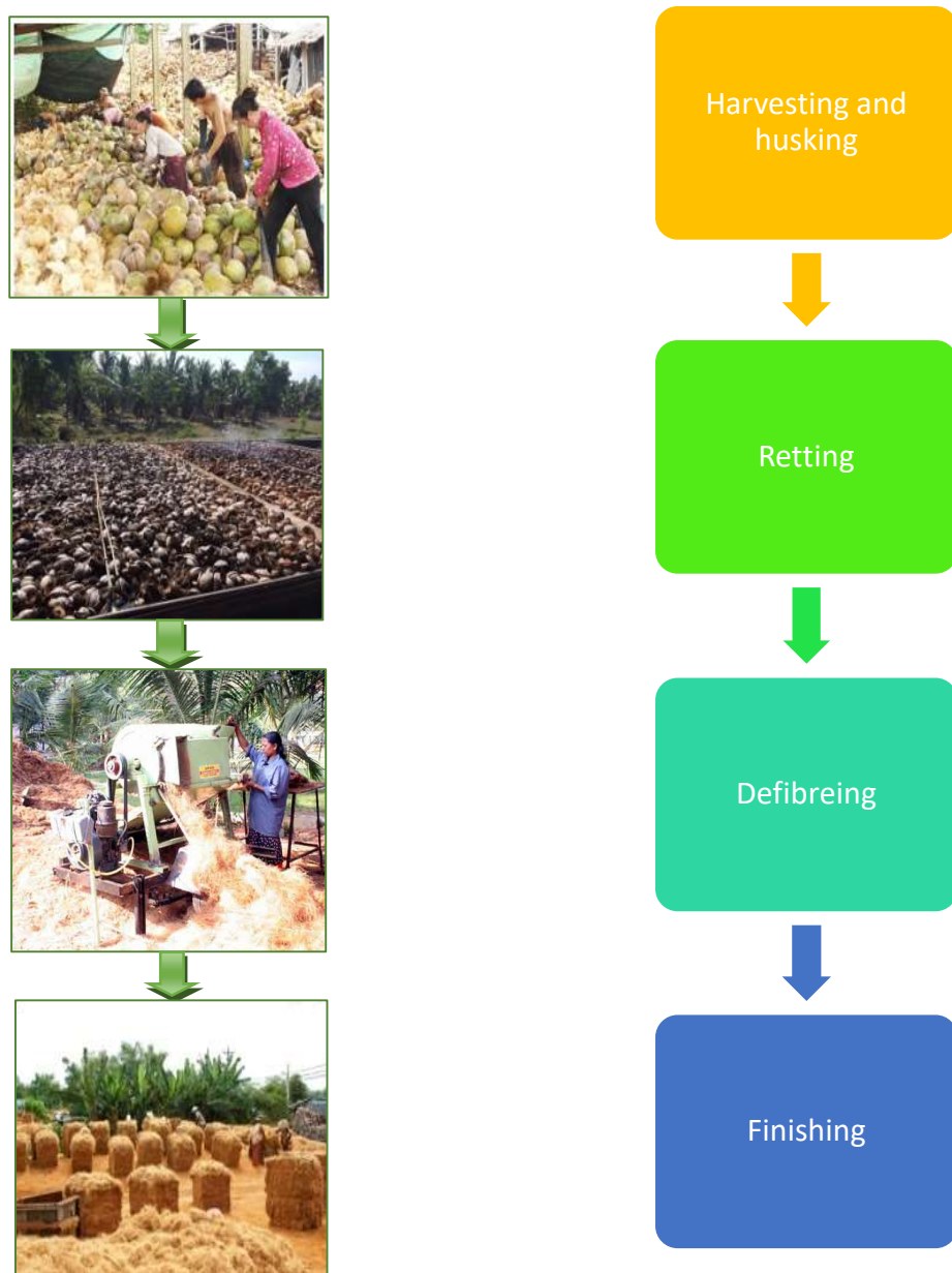
Fig. 1.4. Manufacturing process of coconut fibres.
