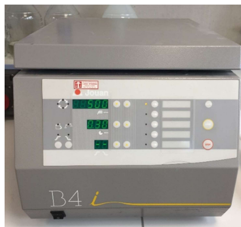
Fig. 3.7. The centrifuge machine installed for water absorption test.
