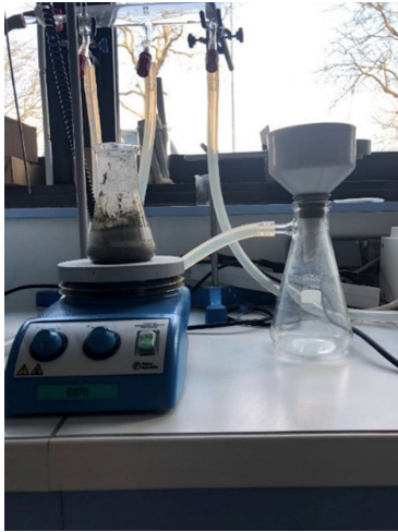
Fig. 2.15. Stirring and filtering powder sample.
