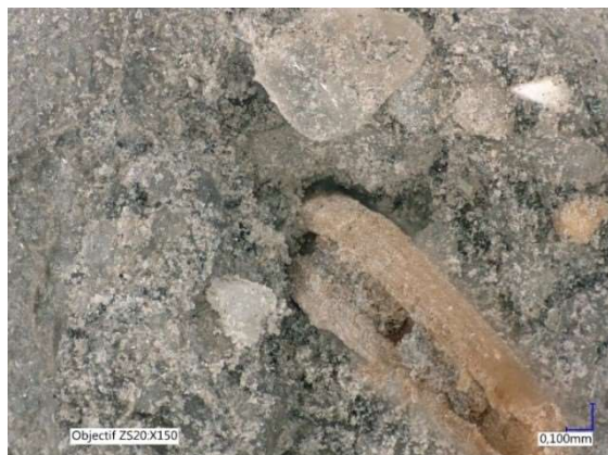
Fig. 3.21. The image of fibre in mortar.
