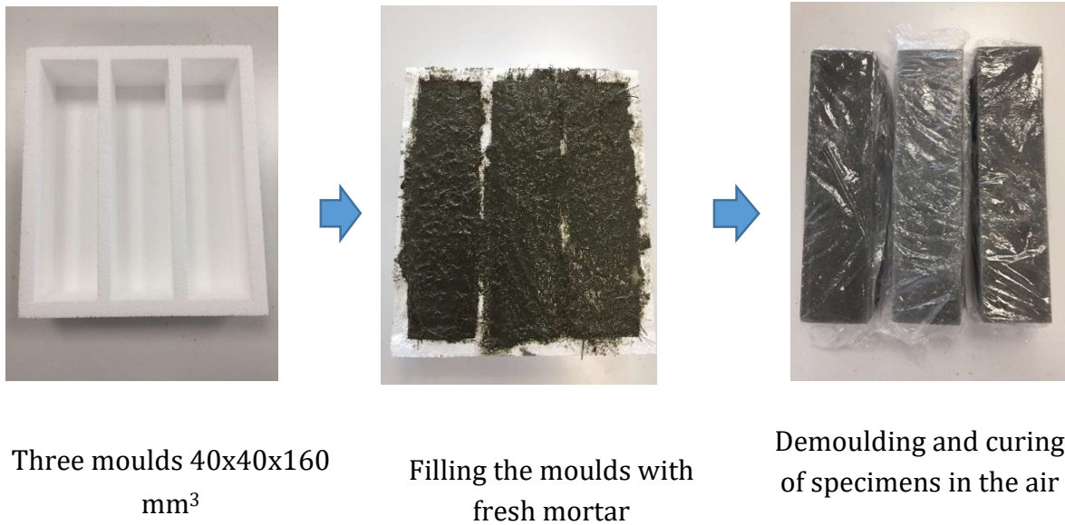
Fig. 2.9. The procedure of casting and curing of samples.
