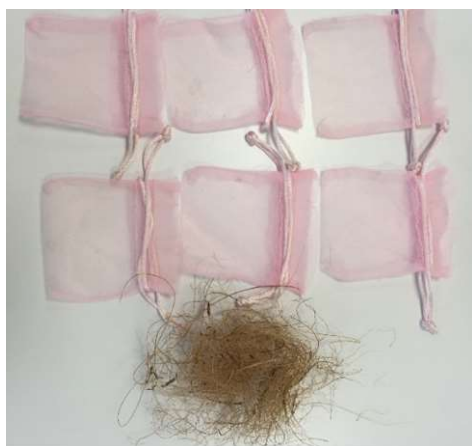
Fig. 3.6. Permeable bags to contain fibres.
