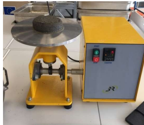
b. Spread out the mortar.
