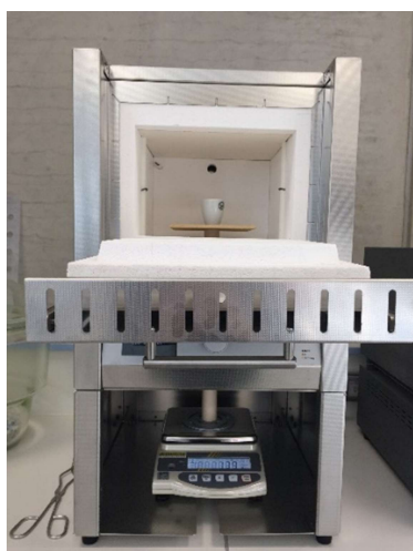
Fig. 3.4. Calcination oven with balance attachment.
