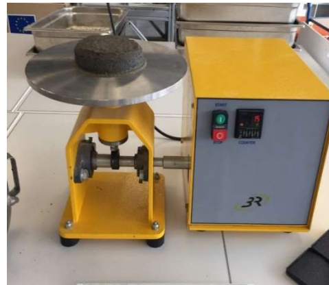
b. Spread out the mortar.
