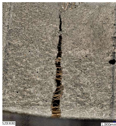
Fig. 4.22. Fibres bridging at the cracked surface of the specimen inclusion of 2% fibre loaded in opposite casting direction.
