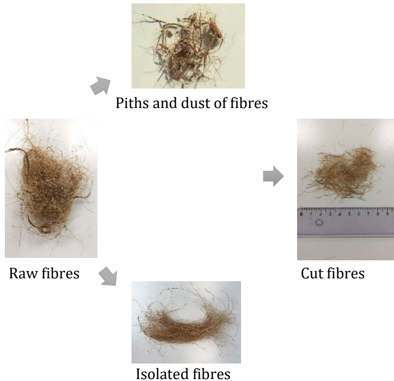
Fig. 2.3. The process of preparation of fibres.
