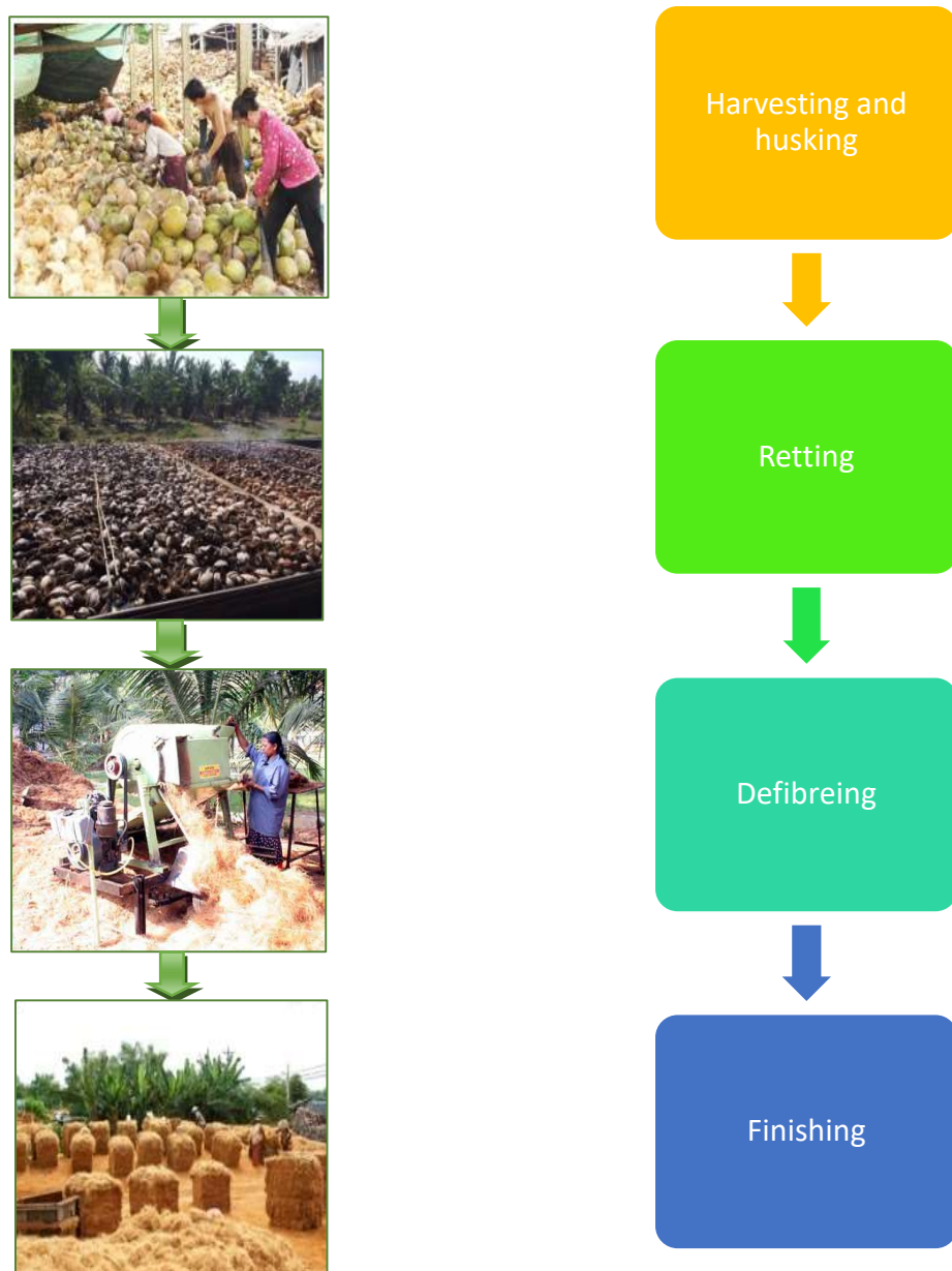
Fig. 1.4. Manufacturing process of coconut fibres.
