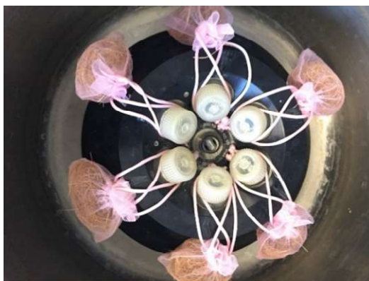
Fig. 3.8. Bags containing fibres put in the centrifuge.
