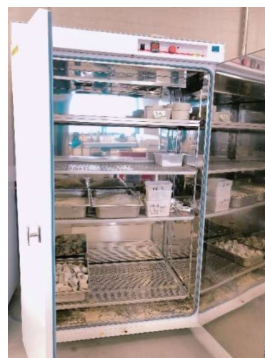
Fig. 3.5. Ventilated oven for drying fibres.
