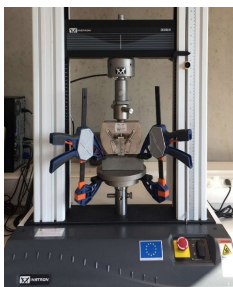
Fig. 3.14. Single fibre pull-out test set up
