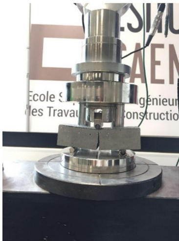
Fig. 2.17. Flexural three points test.
