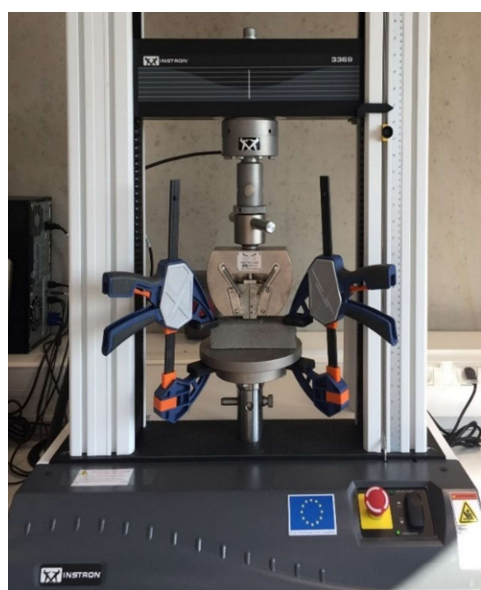
Fig. 3.14. Single fibre pull-out test set up
