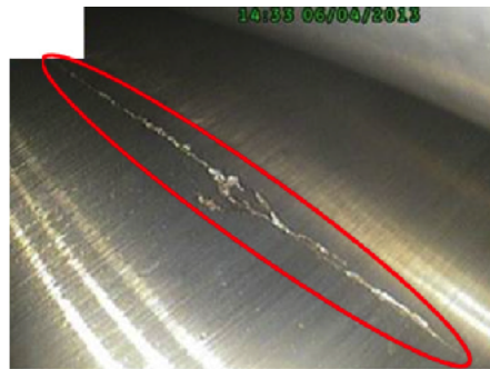
Figure 3-5: Cracked inner race of the high speed shaft bearing after the last day of recording.
