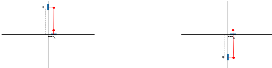
Figure 8.3: The parallel singular poses of \underline{PRRP} where the pose x admits two commands.
