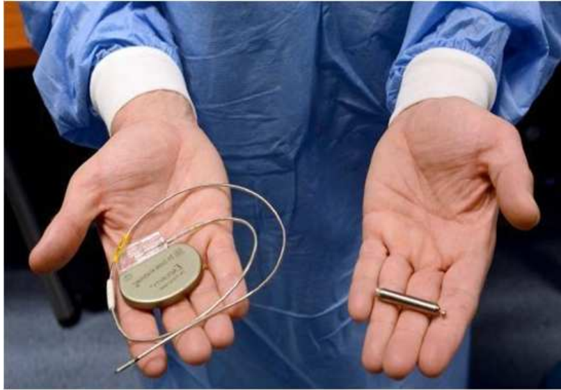
Figure 2.9: Standard Cardiac Pacemaker on the left hand side and Leadless Cardiac Pacemaker (Nanostim, St. Jude) on the right hand side.
