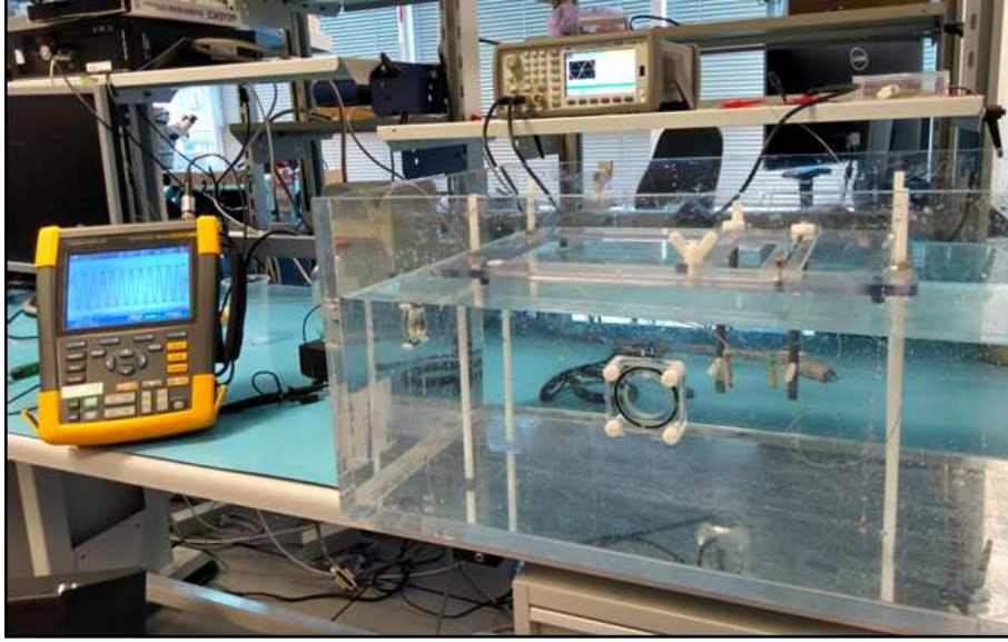
Figure 3.27: Custom phantom used for preliminary verification. Dimension of the tank were 50 cm x 36 cm x 26 cm containing 40 l of solution.
