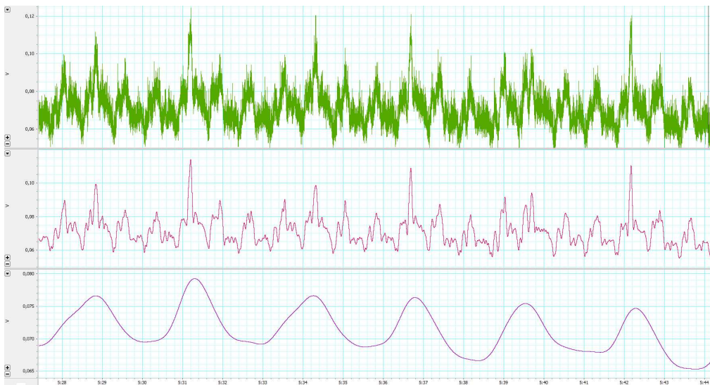
Figure 3.38: Long-time representation of the envelope amplitude. In green the raw envelope signal, in red the envelope signal low-pass filtered at 20 Hz; in purple the envelope signal low-pass filtered at 0.7 Hz
