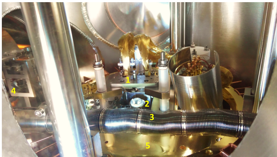
Figure 3.7: Inside view of the surface characterization unit of the multi-probe setup. 1- sample stage, 2- tip holder, 3-UHV wobble stick for sample transfer, 4- sample storage rack, 5- platform for temperature variation
