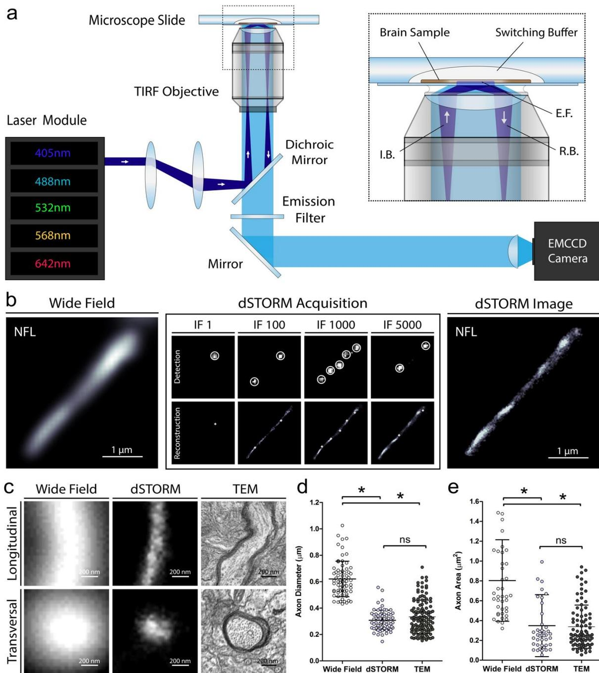
**Fig. 1. Super-resolution imaging of human brain samples.** a, Schematic of the optical setup used for STORM imaging.
