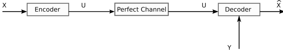
Figure 2.4: Lossless Source Coding with side information
