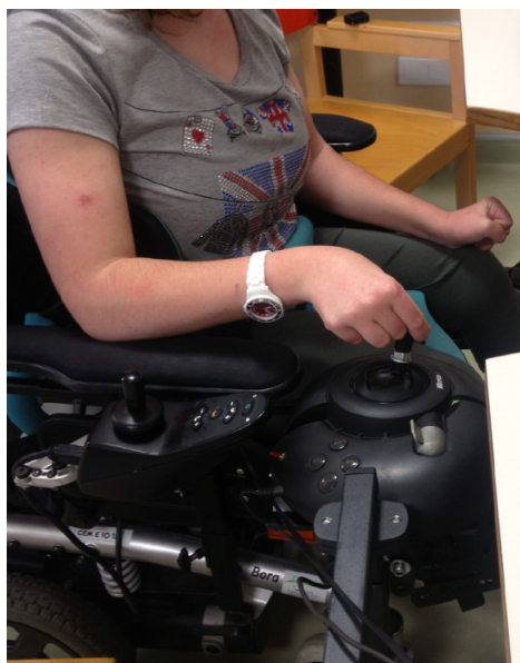
Figure 2.10: Experiment wheelchair with joystick force feedback modified from the Microsoft Sidewinder Force Feedback 2 [36]
