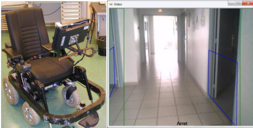
Figure 2.3: Intelligent wheelchair and the interaction screen where the user selects their desired task developed at University of Lorraine, France [17]
