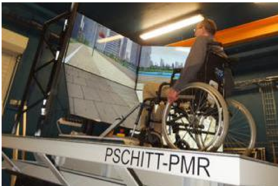
Figure 3.1: Virtual-reality System: PSCHITT-PMR (LAMIH) dynamic interactive platform for wheelchair simulations. It can be used with the manual, powered or hybrid wheelchairs (Hybrid wheelchair is basically a motorized version of manual wheelchair which can operate in both manual and powered mode or even assisted-manual mode).
