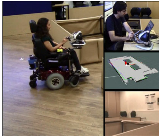
Figure 2.16: Experiment set up in [38] where the remote assistant who is provided with a visualization and real-time camera capture.
