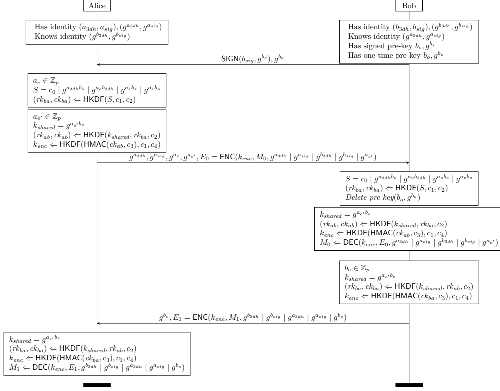
Figure 1.2: SP, a variant of Signal with minor differences. Alice requests a signed pre-key from Bob (via the server) and sends an initial message M_0 . Bob accomplishes his side of the key exchange and obtains M_0 . Bob later sends his reply M_1 , illustrating the Axolotl ratchet post-AKE. We ignore the hash-based ratchet that occurs when two consecutive messages are sent in the same direction. c_i refers to various constants found throughout the protocol.
