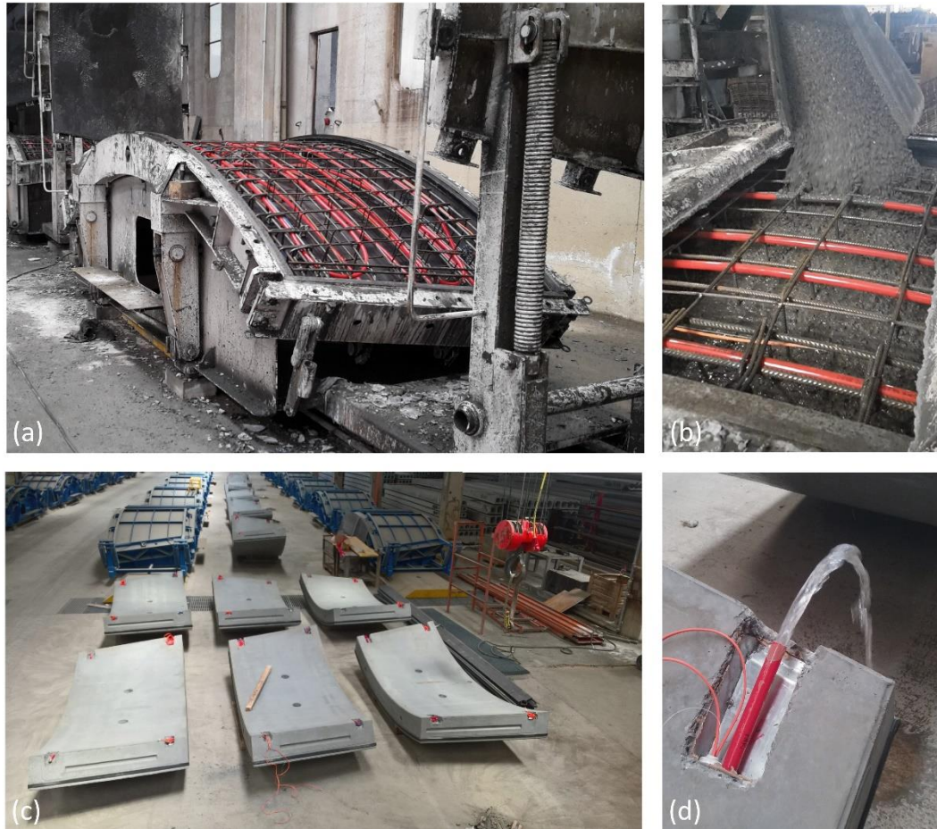
Figure 4.7: Preparation stages of energy segments: (a) moulding, (b) casting, (c) demoulding and (d) circulation test.
