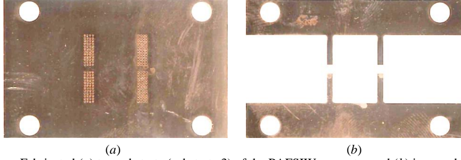
Fig. 3.14. Fabricated (a) top substrate (substrate 3) of the PAFSIW resonator and (b) inner substrate (substrate 2) of the AFSIW iris resonator, with L = 8.418 mm and 8.43 mm for the PAFSIW and AFSIW resonators, respectively.
