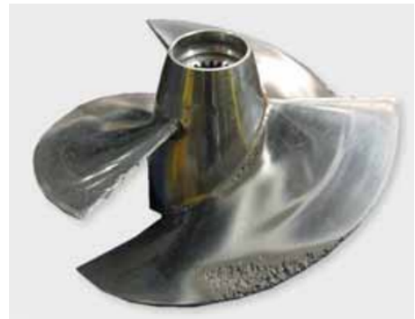
(b) propeller blade destroyed by cavitation erosion.
