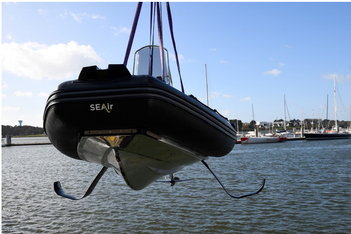
FIGURE 1.5 – SEAIR's flying rib : foiling motor boat with J foil, [109]
