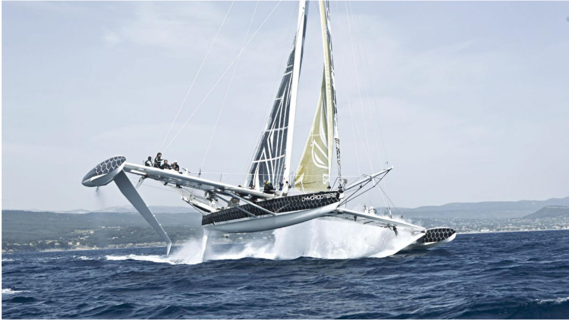
FIGURE 1.6 – Alain THEBAULT's hydrofoil 'Rocket' type I with fences to avoid ventilation. [118]
