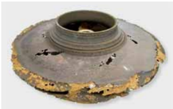
(a) Pump rotor destroyed by cavitation erosion.
