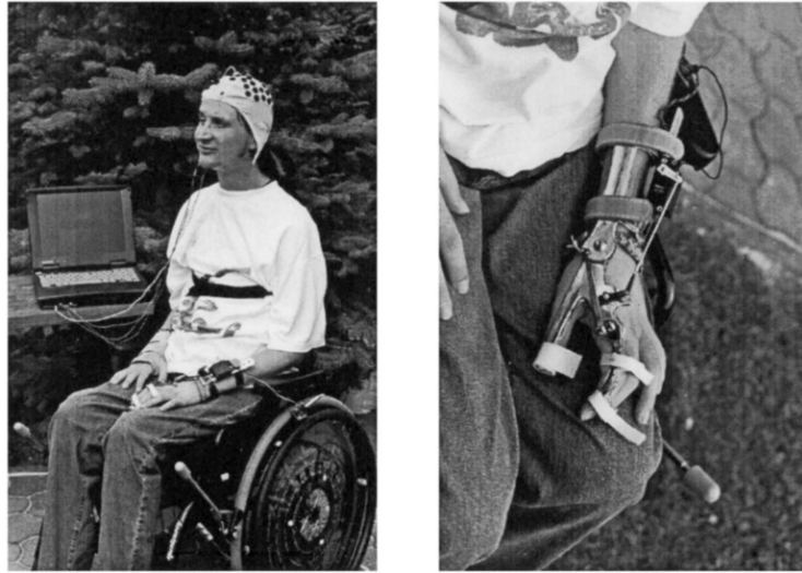
Figure 2: The first hand orthosis introduced in BCI from Pfurtscheller and colleagues [20]. The subject had to imagine a movement of his hand to operate the device, which is directly based on his brain's bioelectric signals.
