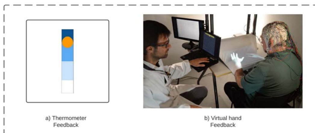
Figure 2.1: Visual feedback used in NF/BCI studies. (a) Activity meter feedback, the ball reflect the subject current level of activity [52]. (b) Virtual Hand that performs the imagined movement on successful trials [105].
