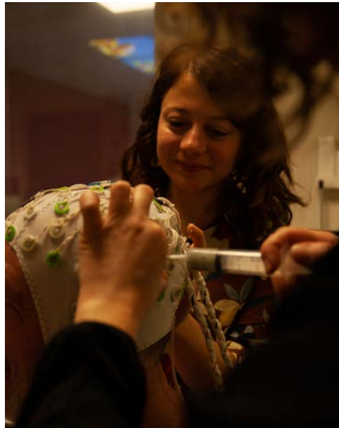
Figure 1.2: Photography of a 64-channel MR-compatible EEG (Brainproduct).
