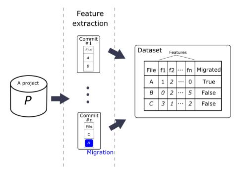
Figure 6.5: The creation of the training dataset for classification. Given *P* and its list of commits with migration, we checkout the source code for each commit. Then, we extract the features for all project files. Later, this information is formatted. In this format, each file becomes a row in the dataset, and each column contains information related to one feature. There is also one column that indicates if that file was migrated or not.
