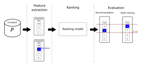
Figure 6.6: For each commit in the training dataset, our approach generates a ranking with all project files. This ranking is compared to an ideal ranking created from the corresponding commit, where the migrated files are in the top. In this example, we set k = 2, so only the first two positions of the rankings are considered in the evaluation.
