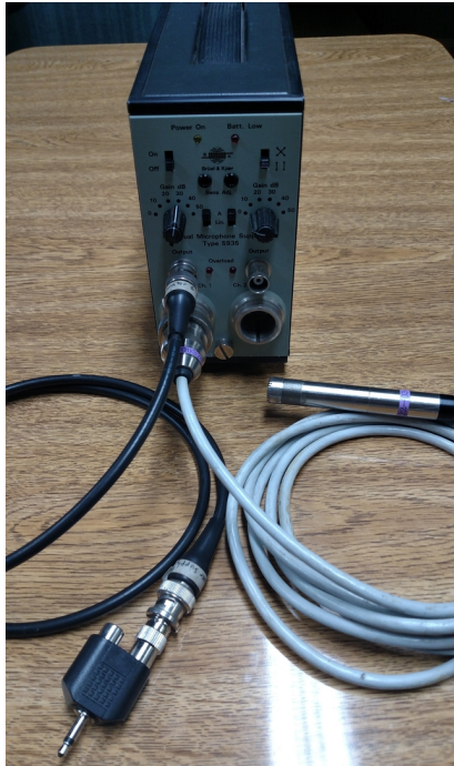
Figure 32 – Microphone Brüel & Kjær for stimuli acquisition.
