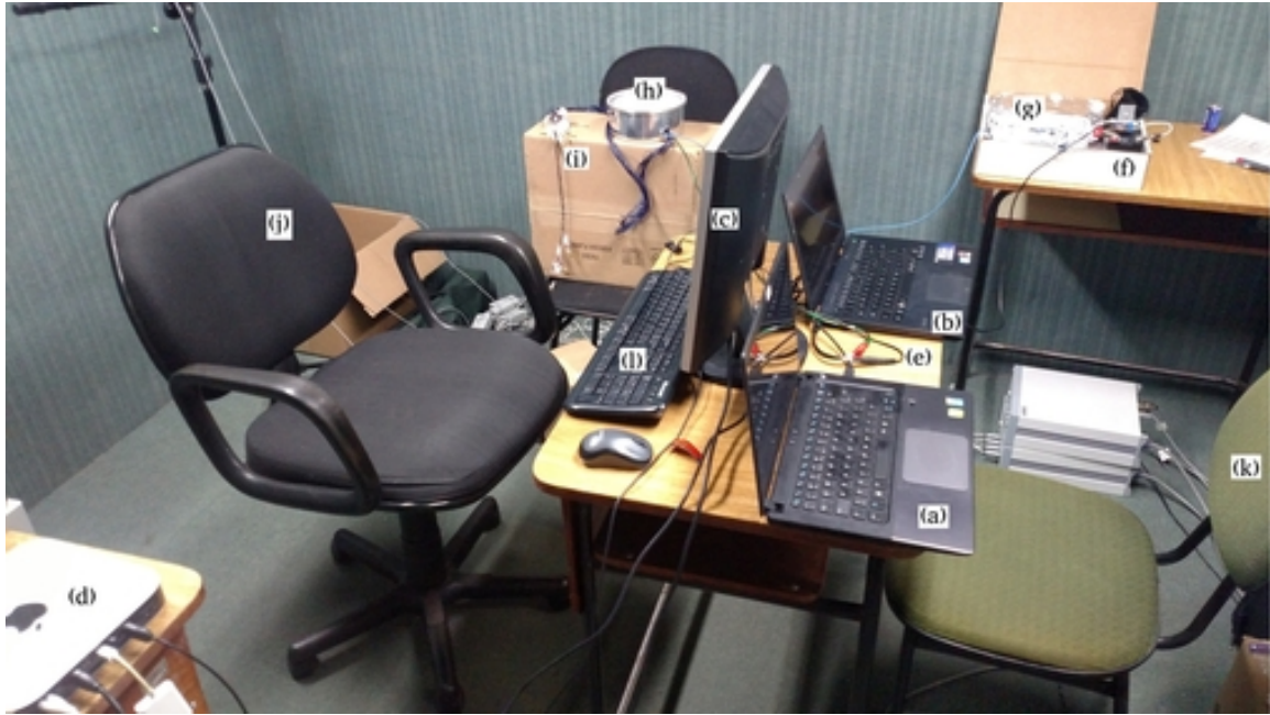
Figure 12 – Room layout for the acquisition protocol adopted. (a) Computer for signals acquisition. (b) Computer for stimuli generation and responses reception in all stages of the protocol. (c) Monitor for participant interaction. (d) Computer to display videos in the passive task. (e) Cable for audio channels separation. (f) Battery to power the RHD2000. (g) RHD2000 evaluation system. (h) RHD2000 amplifier, electrodes connector and optocoupler circuit. (i) Electrodes. (j) Chair for the participant. (k) Chair for the researcher. (l) Keyboard for participant interaction.
