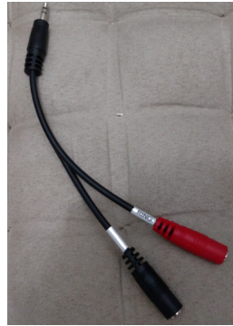
Figure 22 – Cable to separate audio channels.
