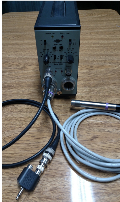
Figure 32 – Microphone Brüel & Kjær for stimuli acquisition.
