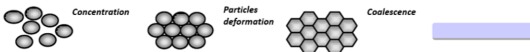
Figure 1.4: Diagram illustrates the three stages of film formation by drying soft particles.
