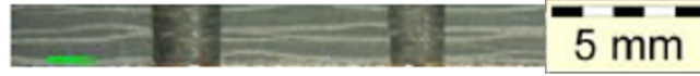
FIGURE 1.3: Cross-sectional view of a perforated plate with R_{\text{neck}} = 0.9 mm. Note that this view does not intersect with both of the perforations axes.
