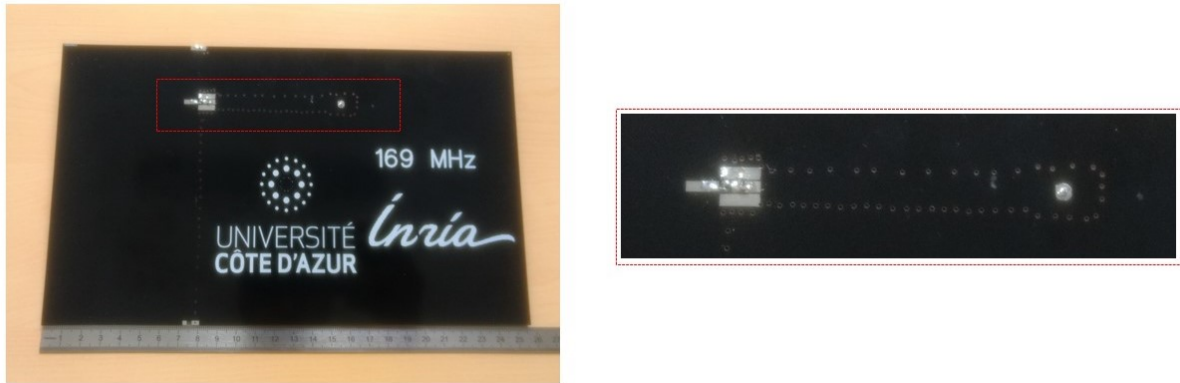
Figure 5.17: 169 MHz PCB Antenna with 5 component matching circuit
