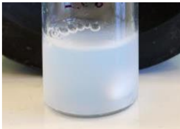
Figure II.33. The final solution picture resulting from UV-light initiated RAFT-PITSA of NAGA using Photo-I as photoinitiator and Thermal-PPEGA 24 as macro-CTA in aqueous dispersion at 5 °C.
