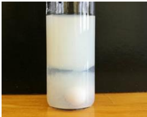
Figure III.5 Picture of the reaction medium obtained after 30 min of a UV-light initiated RAFT-PITSA of NIPAm/MBA mediated through photo-I and UV-PPEGA 18 ( [\text{NIPAm}]_0/[\text{MBA}]_0/[\text{UV-PPEGA}_{18}]_0/[\text{Photo-I}]_0 = 204/8/1/0.3 ) with a solid content of 2.4 wt.% in water at 70°C.
