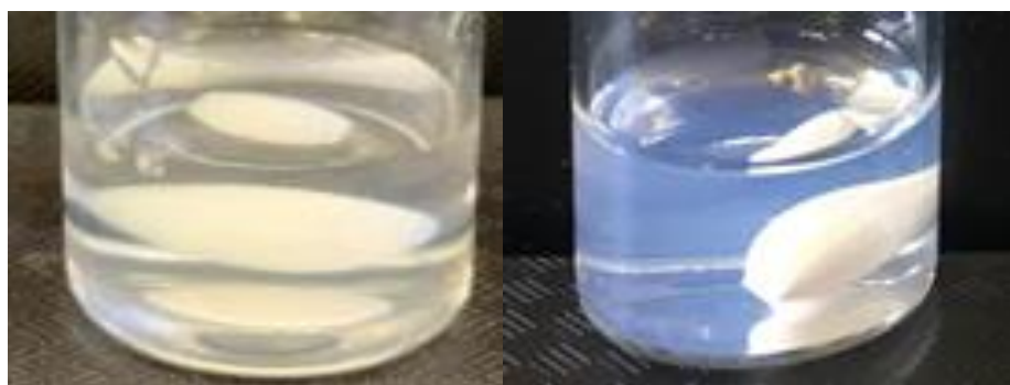
Figure IV.2. Picture of the reactional medium of UCST-1 before and after 1h of UV-light initiated RAFT PITSA of NAGA/MBA using Thermal-PPEGA 30 in water at 3°C. Initial molar ratio: [Thermal-PPEGA 30 ] 0 /[NAGA] 0 /[MBA] 0 /[Photo-I] 0 =1/400/16/0.3 with a solid content of 2.4 wt.%.
