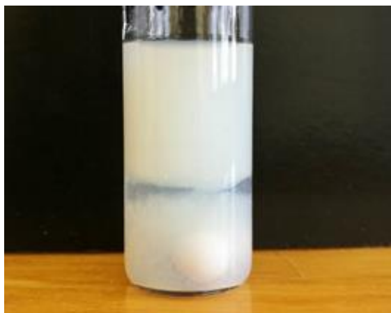
Figure III.5 Picture of the reaction medium obtained after 30 min of a UV-light initiated RAFT-PITSA of NIPAm/MBA mediated through photo-I and UV-PPEGA 18 ( [\text{NIPAm}]_0/[\text{MBA}]_0/[\text{UV-PPEGA}_{18}]_0/[\text{Photo-I}]_0 = 204/8/1/0.3 ) with a solid content of 2.4 wt.% in water at 70°C.
