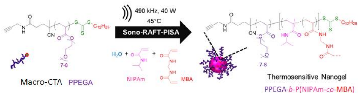
Figure I.43. Synthesis of LCST-type thermosensitive nanogels based on PPEGA- b -P(NIPAm- co -MBA) via Sono-RAFT-PITSA process. Reproduced from ref.148
